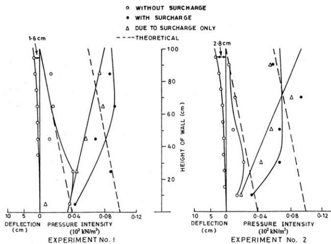
Figure 3: Pressure Distribution and Deflected Position of Model Wall. (Measured on Perspex Sheet)
