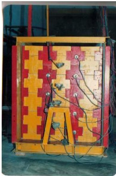
Figure 2: The positions of dial gauges and pressure cells
