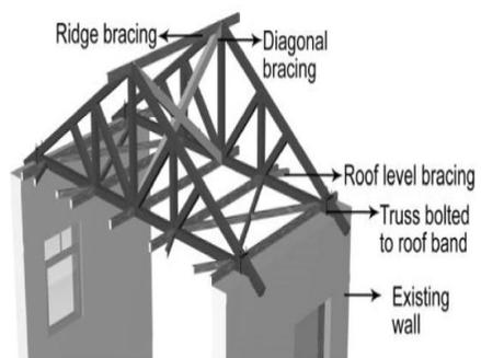
Figure 12: Bracing of sloped roof (IIT Roorkee, 2006)
