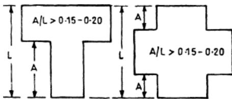
Figure 1: Example of Re-entrant corner (IS 1893 Part 1:2002)
