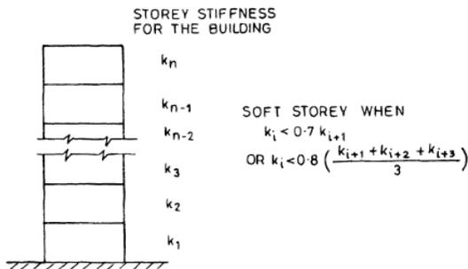
Figure 5: Stiffness irregularity (IS 1893 Part 1:2002)
