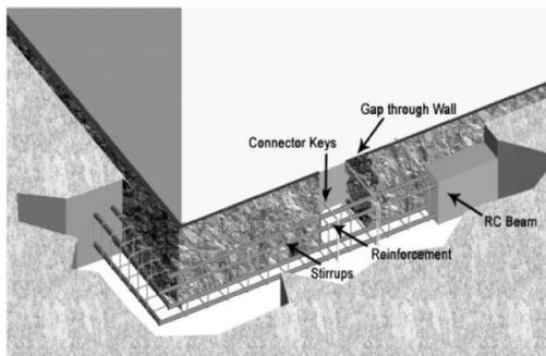
Figure 11: Strengthening of foundation (IIT Roorkee, 2006).
