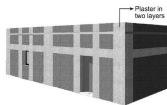
Figure 10 : Plastering of nailed wire mesh (IIT Roorkee, 2006)
