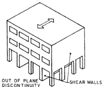
Figure 3: Out of plane offsets (IS 1893 Part 1:2002)
