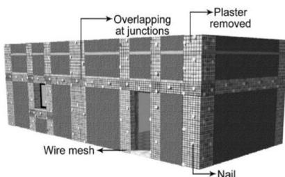
Figure 9: Nailing of wire mesh (IIT Roorkee, 2006)
