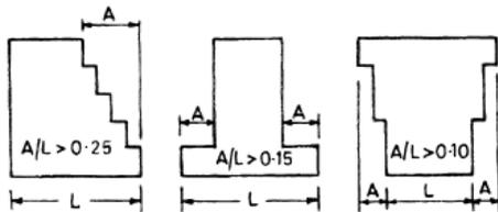
Figure 7: Vertical geometric irregularity (IS 1893 Part 1:2002)
