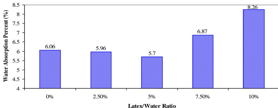
Figure 2: Effect of latex dosage on Water Absorption
