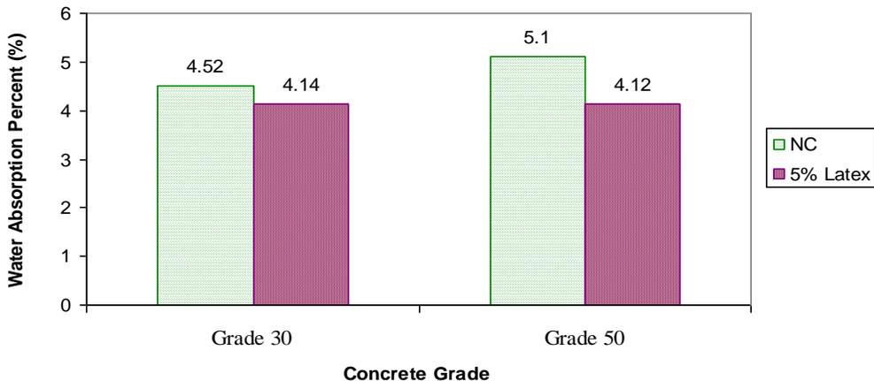
Figure 3: Effect of concrete grade on Water Absorption
