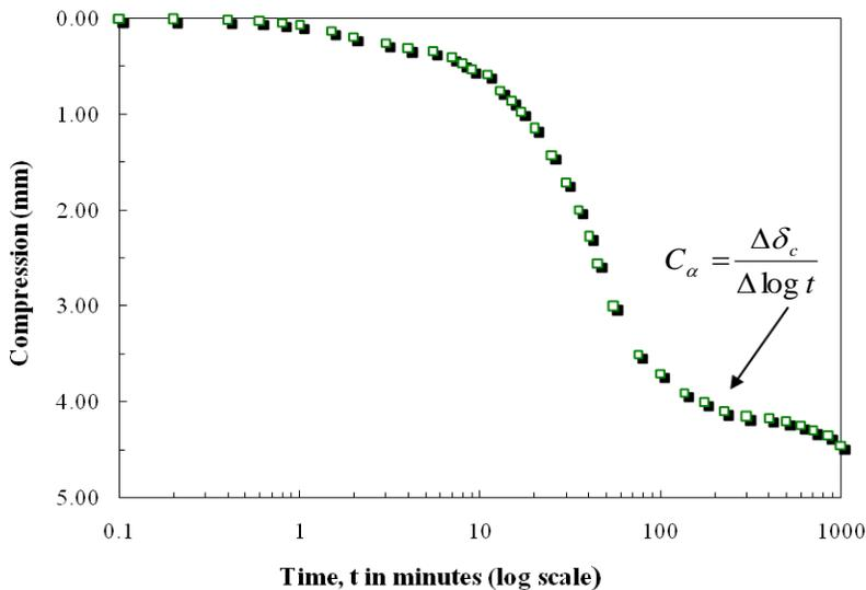
Figure 3: Typical time compression curve from consolidation test
