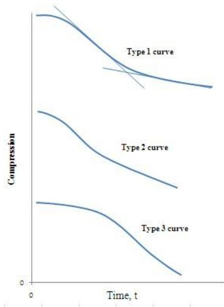
Figure 1: Types of compression versus logarithmic of time curve derived from consolidation test (Leonards and Girault, 1961)
