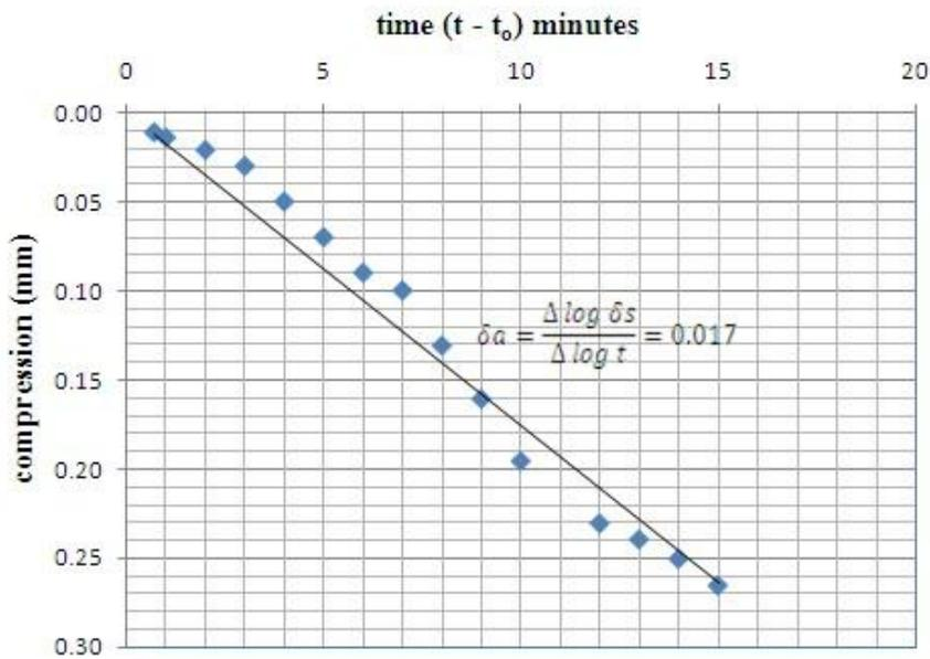
Figure 7 : Determination of index of secondary consolidation ( $\delta_s$ )
