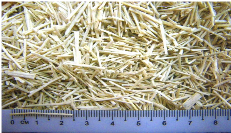
Figure 1: Cut and treated oil palm stem fiber.
