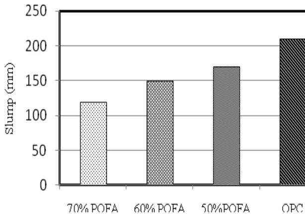
Figure 3: Slump of HVPOFA concrete at 0.48 W/C
