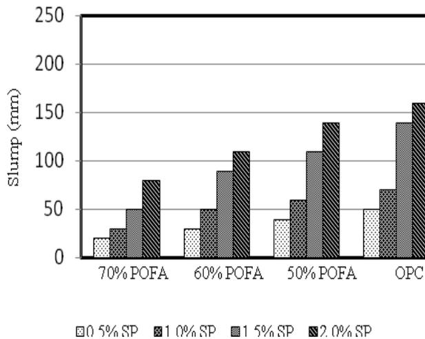
Figure 4: Slump of HVPOFA concrete at 0.42W/C
