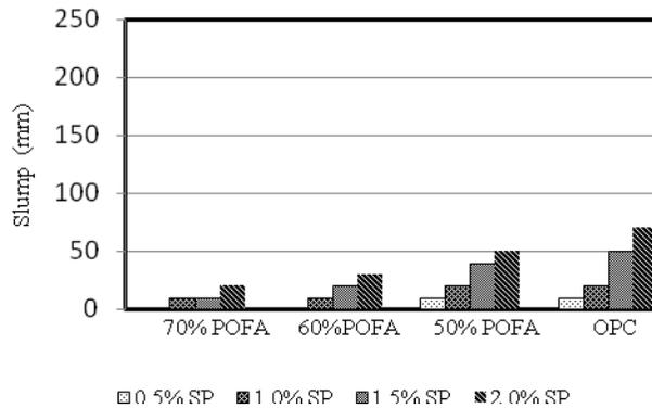
Figure 5: Slump of HVPOFA concrete at 0.38 W/C
