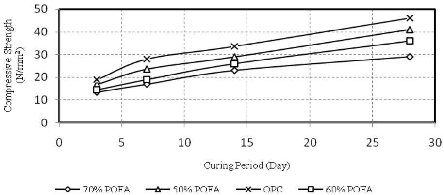
Figure 7: Compressive strength of POFA concrete at 0.42 W/C
