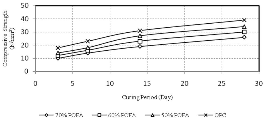
Figure 8: Compressive strength of POFA concrete at 0.38 W/C
