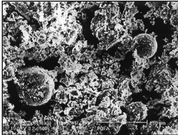
Figure 1: Scanning electron microscope of POFA
