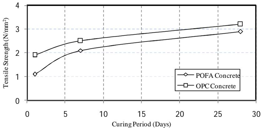
Figure 10: Development of tensile strength in OPC concrete and high volume POFA concrete.
