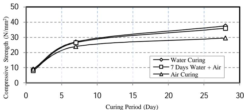
Figure 9: Effect of curing condition on compressive strength of high volume POFA concrete.
