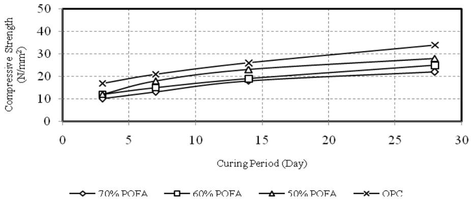
Figure 6: Compressive strength of POFA concrete at 0.48 W/C
