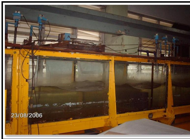
Figure 3 : Wave probe arrangement
