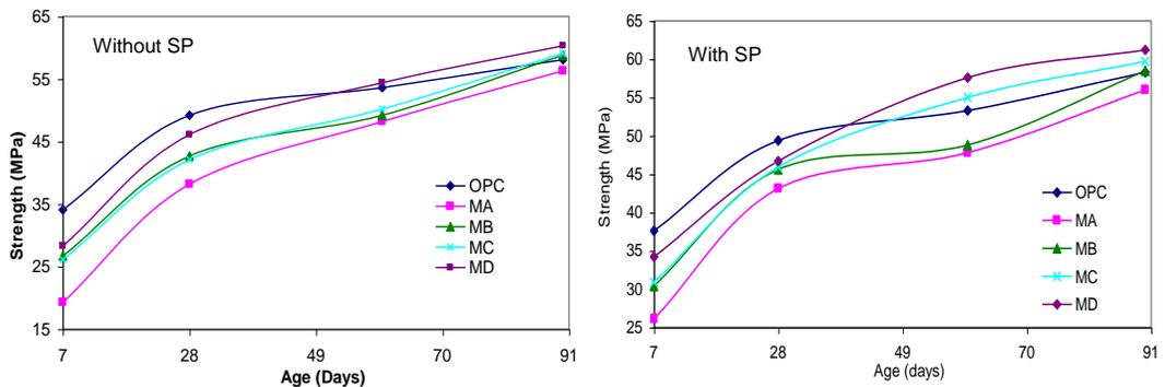
Figure 4: Compressive strength of MBC mortars at different age
