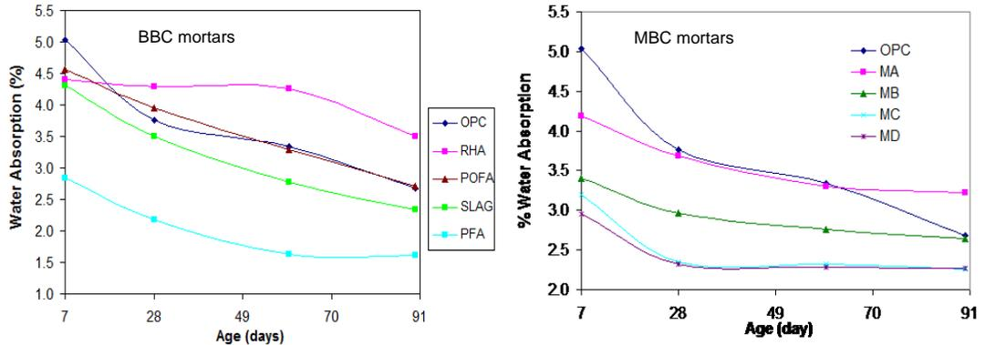
Figure 1: Water absorption of BBC and MBC mortars
