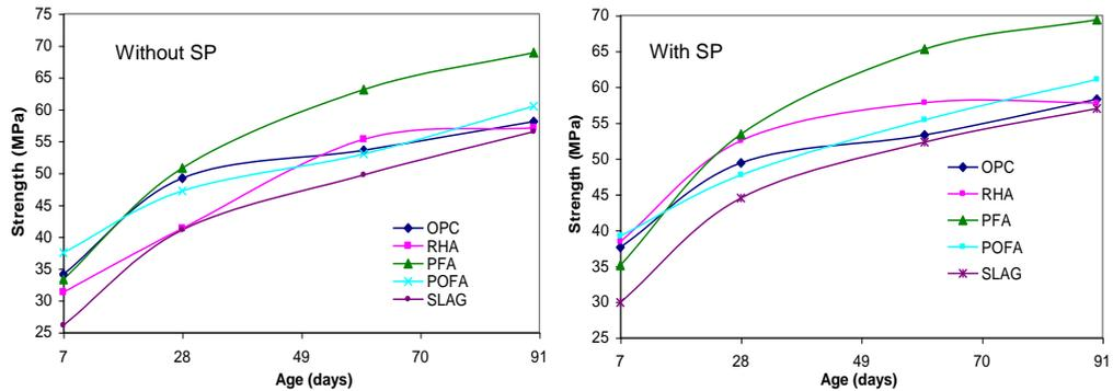
Figure 3: Compressive strength of BBC mortars at different age
