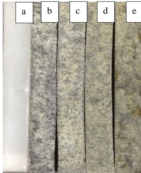
Figure 3: Flexural samples after 32 weeks of outdoor weathering (a) vHDPE, (b) rHDPE, (c) 10 wt% PCB, (d) 30 wt% PCB, (e) 50 wt% PCB
