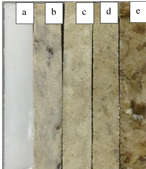
Figure 1: Flexural samples before weathering (a) vHDPE, (b) rHDPE, (c) 10 wt% PCB, (d) 30 wt% PCB, (e) 50 wt% PCB
