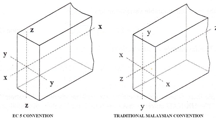
Figure 4: Flexural member axes according to EN 1995-1-1 (McKenzie, 2000).
