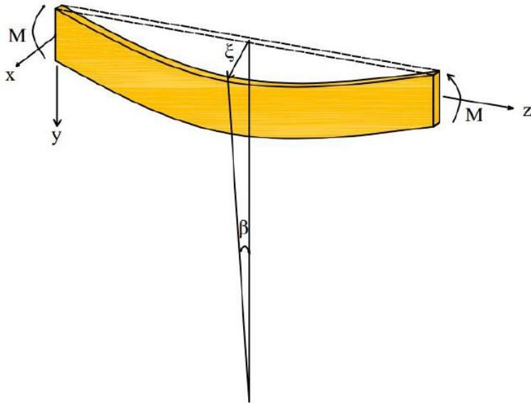
Figure 2: Lateral torsional buckling in timber beams. Notice that the beam has experienced an out-of-plane displacement,  $\xi$ , and has twisted by an angle  $\beta$  (Xiao, 2014).
