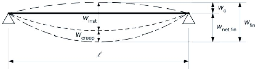
Figure 5: Components of deflection according to EN 1995-1-1.
