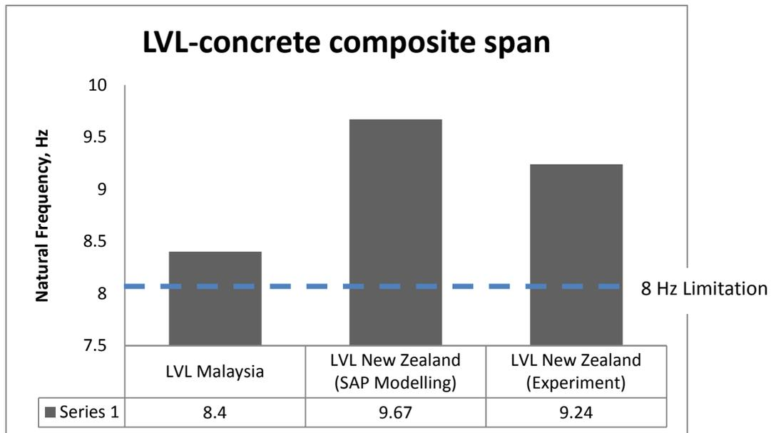
Figure 7: Parameter comparison on LVL-concrete composite span
