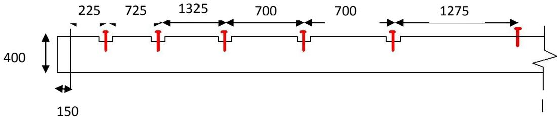
Figure 4: Position of notches and coach screw applied in FE modal 8m span
