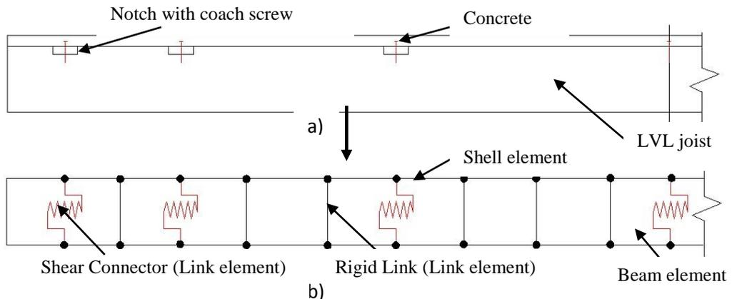
Figure 5: a) Actual span specimen side view b) Beam and shell elements with shear connectors and rigid links
