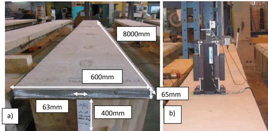
Figure 2: (a) Experimental specimen from previous study [6] (b) electrodynamic shaker used to produce vibration in experiment [6]
