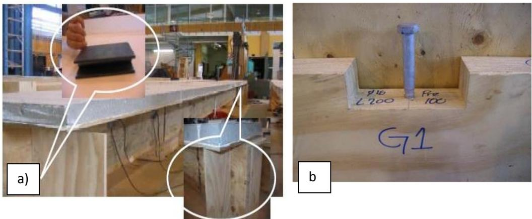
Figure 3: (a) Solid timber block at one end and solid steel roller at the other end of the beam [6] (b) Notch and coach screw on the LVL joist [6]
