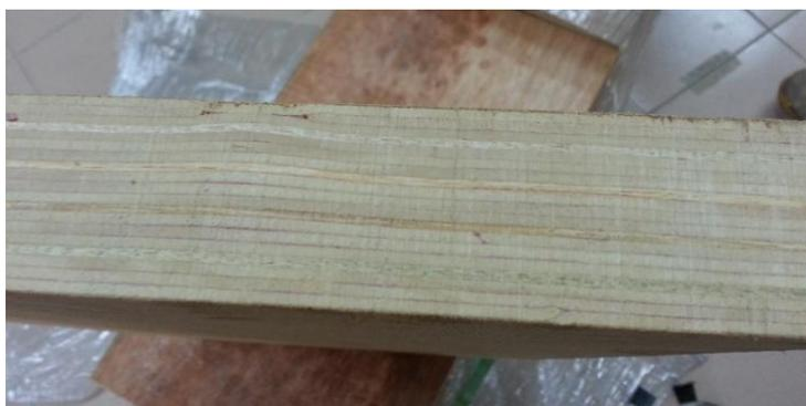
Figure 1: Sample of LVL produced in Malaysia
