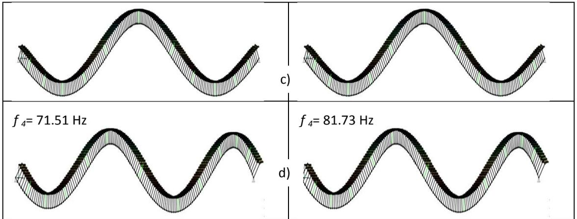
Table 2(cont'): Comparison of the first six mode shapes of LCC beam using LVL from Malaysia (left) and from New Zealand (right)
