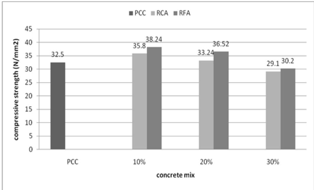
Figure 1: Effect of recycled aggregate on compressive strength of concrete
