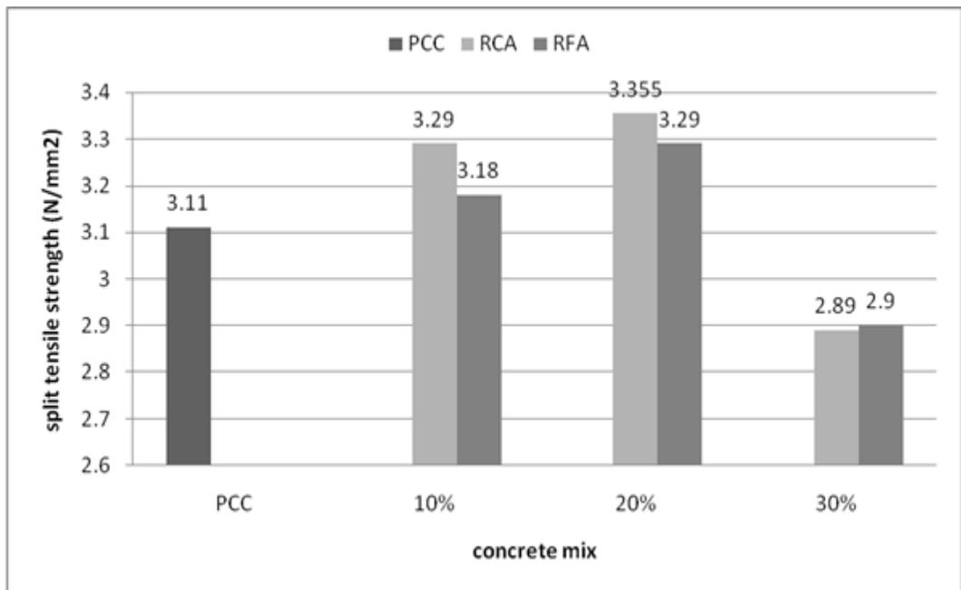
Figure 2: Effect of recycled aggregate on split tensile strength of concrete
