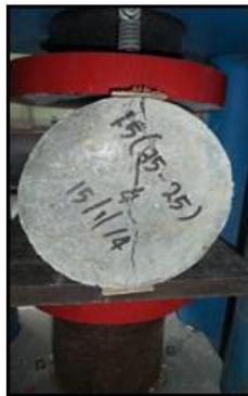
(b) Splitting tensile test
