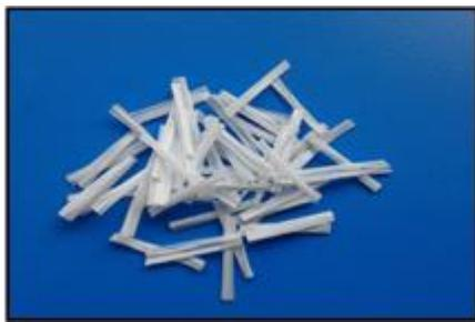
(a) Fibrillated polypropylene fibre
