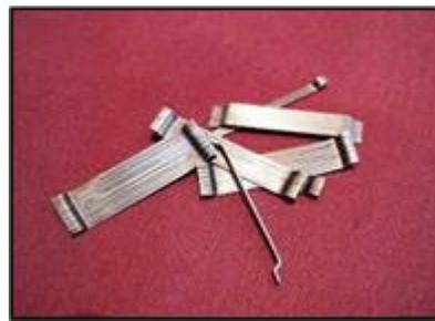
(b) Hooked end steel fibre
