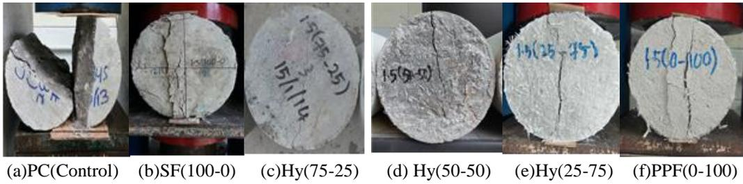
Figure 9: Failure mode of the cylinder specimens
