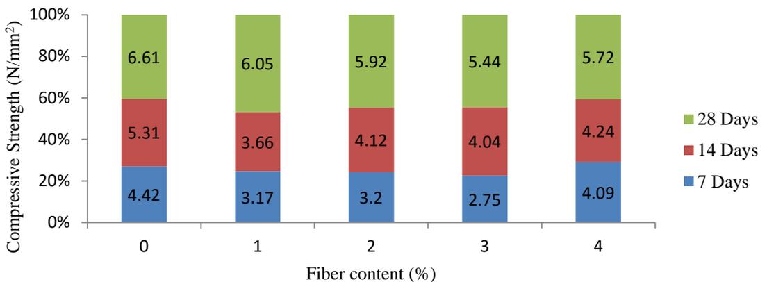
Figure 7: Variation of fiber content with Compressive strength of masonry blocks reinforced with PPF.
