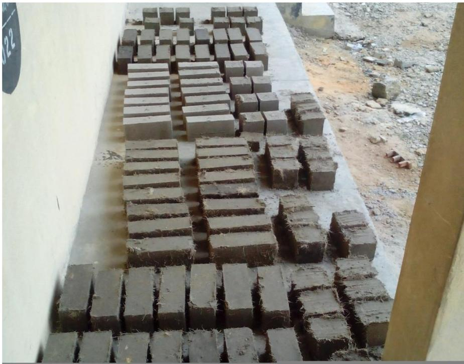
Figure 4: Wet block specimens after casting
