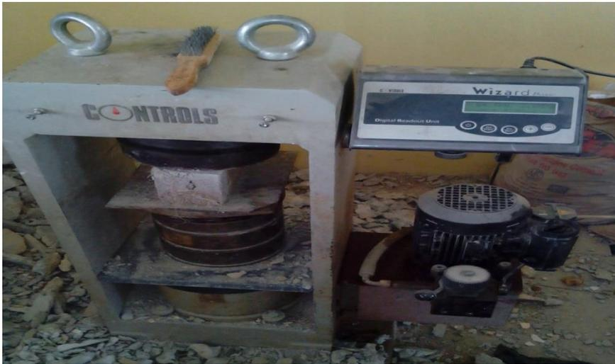
Figure 5: Compressive strength testing of block specimens
