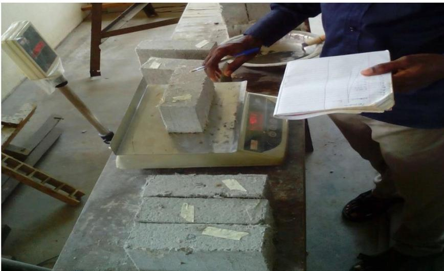
Figure 6: Weighing of Block Samples for Density Determination
