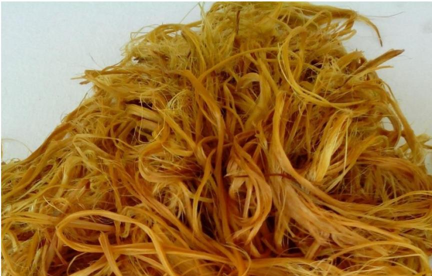
Figure 1: Fiber after being treated in chemical solutions and washed in water.
