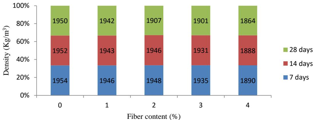
Figure 9: Variation of fiber content with density of masonry blocks reinforced with PPF
