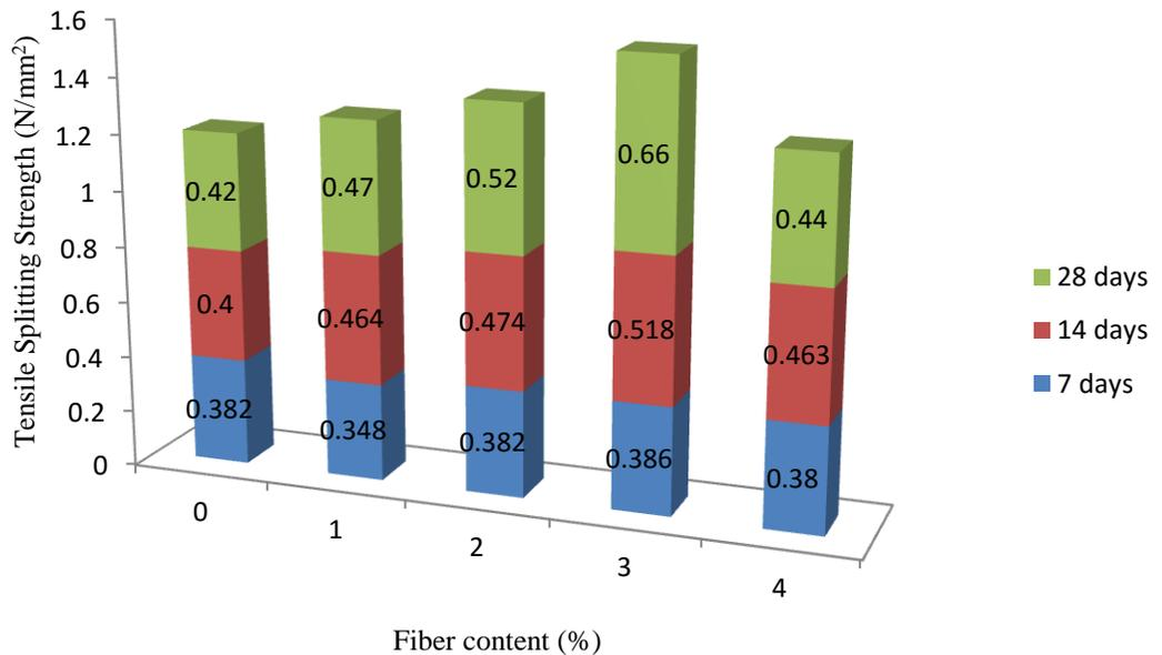
Figure 8: Variation of fiber content with Tensile splitting strength of masonry blocks reinforced with PPF.
