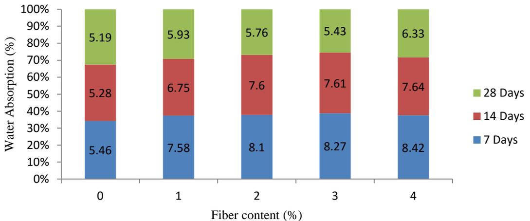
Figure 10: Variation of fiber content with water absorption of masonry blocks reinforced with PPF
