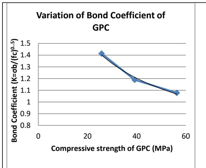
Figure 5: The bond Coefficient (K) of Geopolymer concrete
