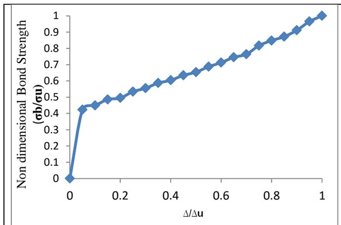
Figure 7: Non dimensional Bond Strength vs slip.
