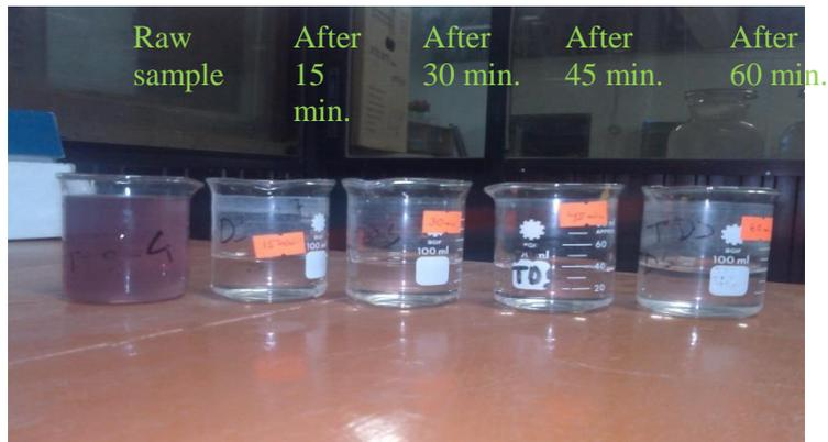
Figure 7: Color of raw sample and samples at different treatment times.
