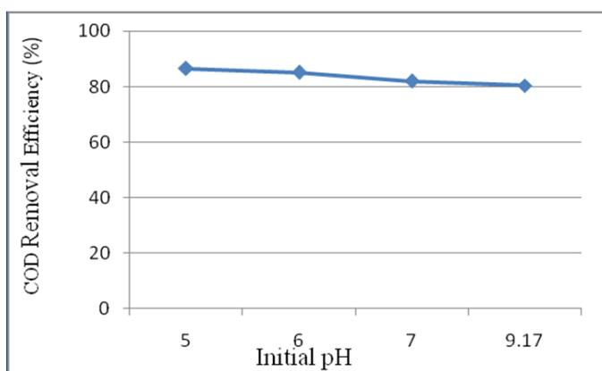
Figure 2: Effect of initial pH on COD removal efficiency after 60 min. of electrolysis.
