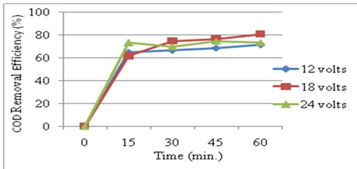
Figure 4: Effect of electrolysis time on COD removal at different electrical potential with the initial pH of raw wastewater
