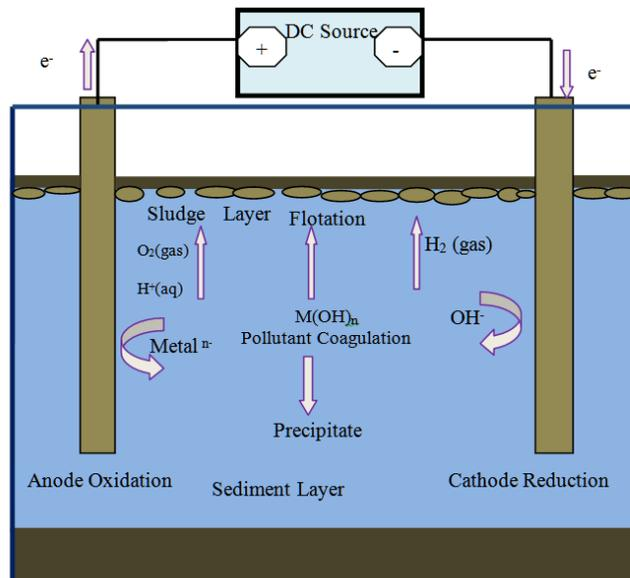
Figure 1: Schematic Diagram of Electrocoagulation Cell
