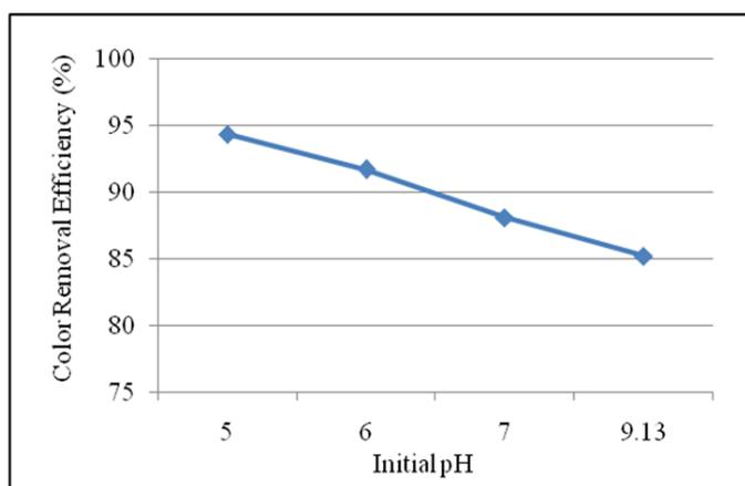
Figure 3: Effect of initial pH on Color efficiency after 60 min. of electrolysis.
