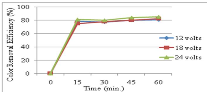
Figure 5: Effect of electrolysis time on Color removal at different electrical potential with the initial pH of raw wastewater
