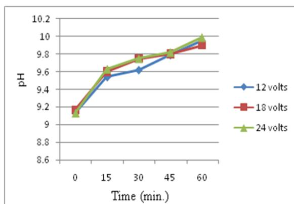
Figure 8: Effect of electrolysis time on pH at different electrical potential
