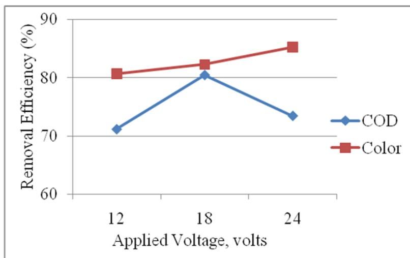
Figure 6: Effect of applied voltage on COD and color removal after 60 min. of electrolysis time
