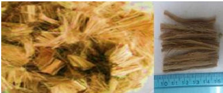
Figure 1: Treated Kenaf fibre chopped to 50mm length
