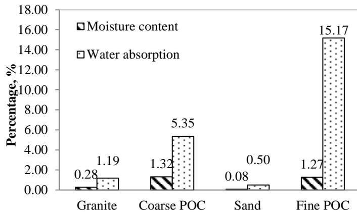
Figure 7: Water absorption and moisture content of POC aggregates
