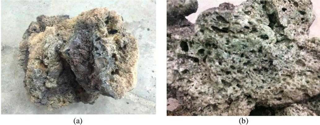
Figure 1: Palm oil clinker, POC (a) POC boulder (b) Porous structure of POC
