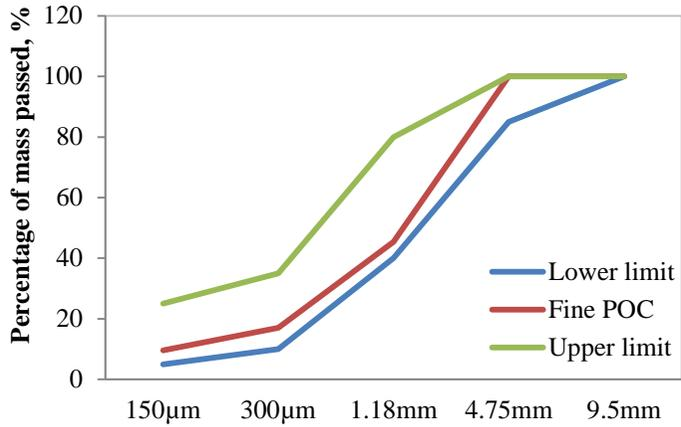
Figure 5: Sieve analysis of fine POC aggregates
