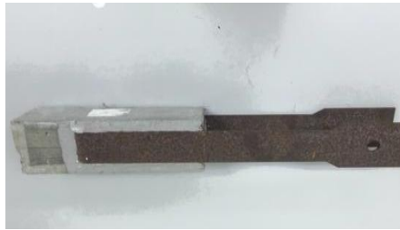
Figures8: SPECS-7 with corroded steel plate
