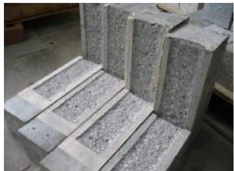
Figure 4: Readily hacked concrete surface
