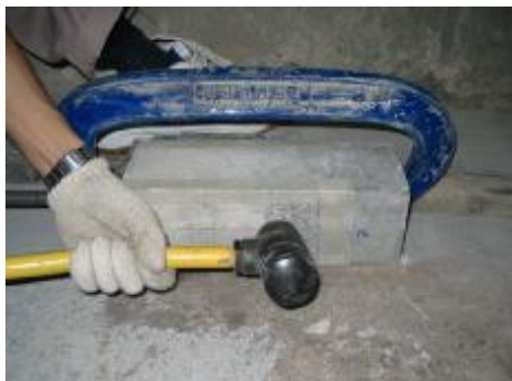
Figure 3: Hacking with air tool hammer
