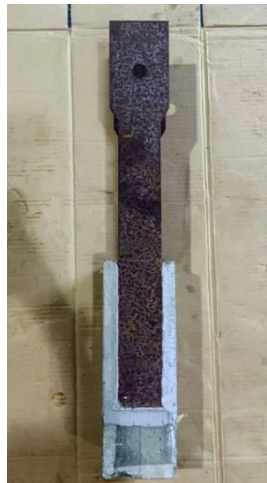
Figure 9: SPECS-7 before the application of rust remover
