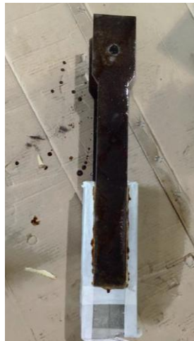
Figure 10: SPECS-7 after the application of rust remover
