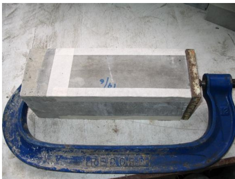
Figure 1: Concrete prisms attached with G-clamp prepared in 2008
