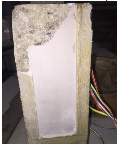
Figure 28: Concrete from SPECS-7 after failure
