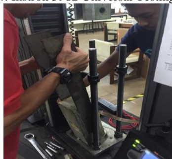
Figure 15: Installation of pull-out test rig
