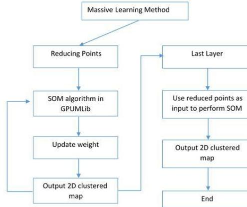
**Figure 3.1** Multilayer SOM flow
