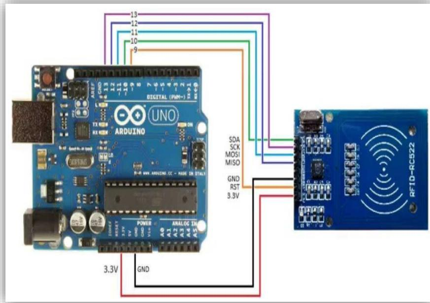
**Figure 2** Connection Diagram Between Arduino Uno and RC522 Sensor
