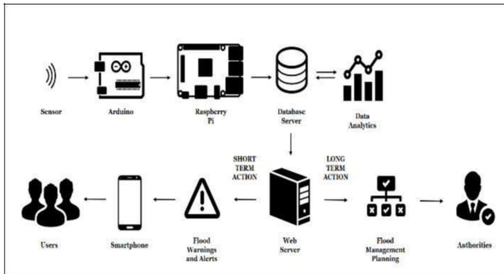
**Figure 2.** Over of the system architecture
