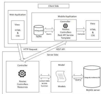
Figure 3 DES system architecture
