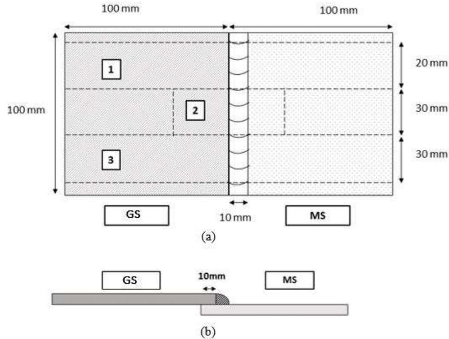
**Figure 1:** Dimensions of the welding plates
