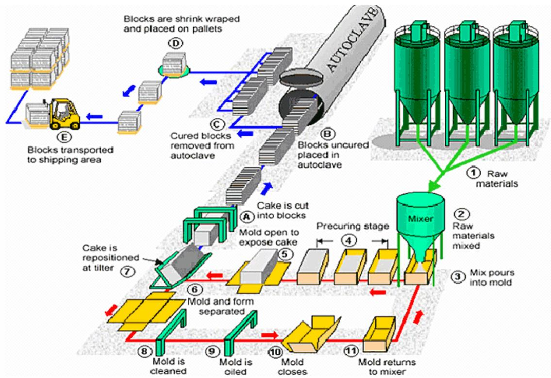
**Figure 2.2** Manufacturing Process of AAC Masonry Units ([www.aacstructures.com](http://www.aacstructures.com))
