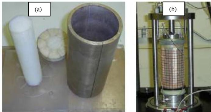
Figure 5: (a) Mold assembly for sample preparation (b) specimen placed in hollow cylinder triaxial cell
