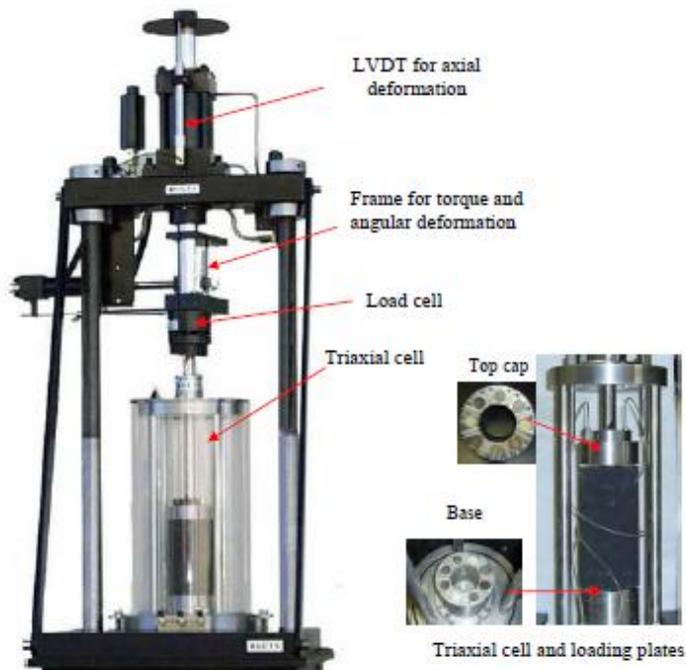
Figure : Loading frame and triaxial cell for HCA
