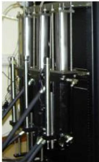
Figure 3: Pressure system for hollow cylinder apparatus
