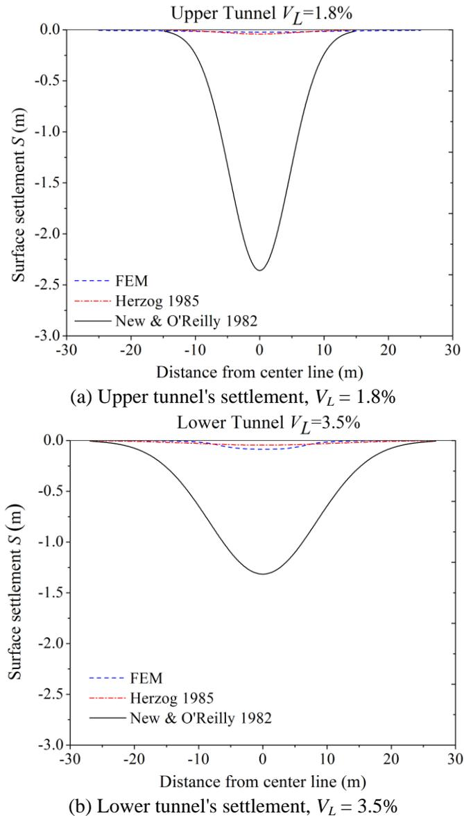
Figure 5: Surface settlement analysis for the study cross-section
