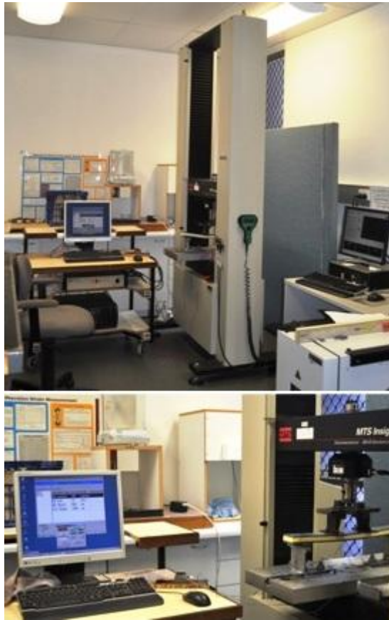
Figure 3: Testing set-up for four point bending test
