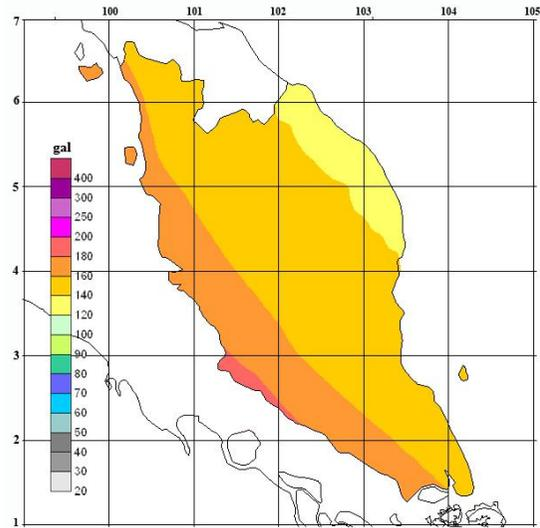
Figure 10. Probabilistic seismic hazard map of 0.2 sec spectral acceleration expected at 10% probability in 50 years on bedrock
