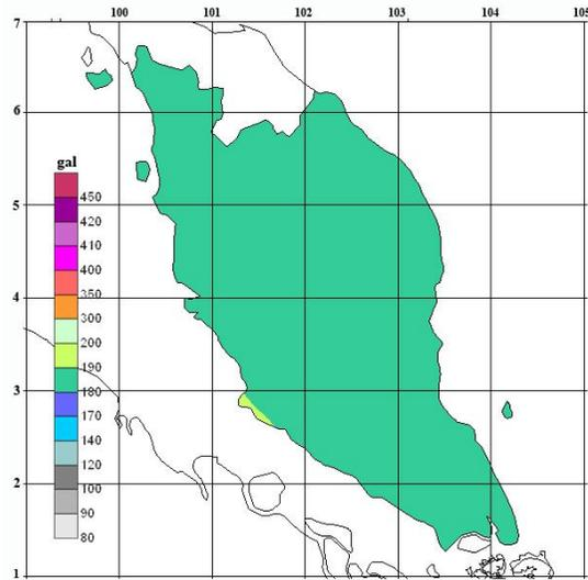
Figure 12. Probabilistic seismic hazard map of peak ground acceleration expected at 2% probability in 50 years on bedrock
