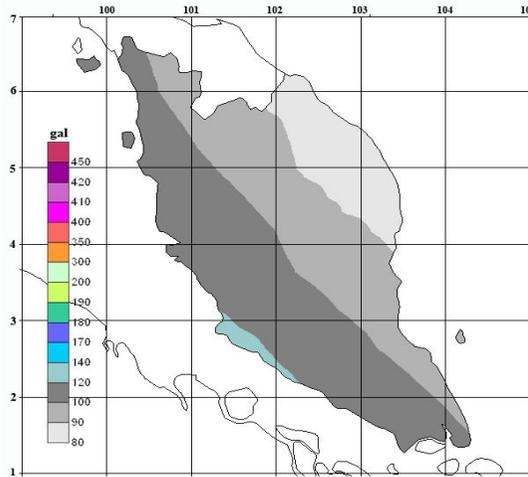
Figure 14. Probabilistic seismic hazard map of 1.0 sec spectral acceleration expected at 2% probability in 50 years on bedrock
