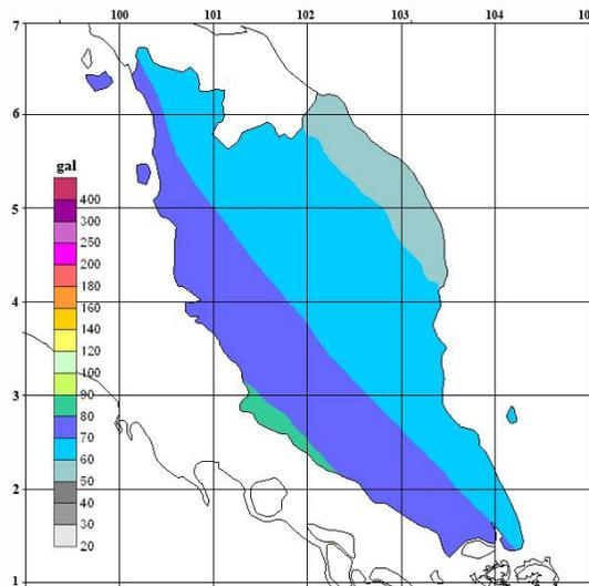
Figure 9. Probabilistic seismic hazard map of peak ground acceleration expected at 10% probability in 50 years on bedrock
