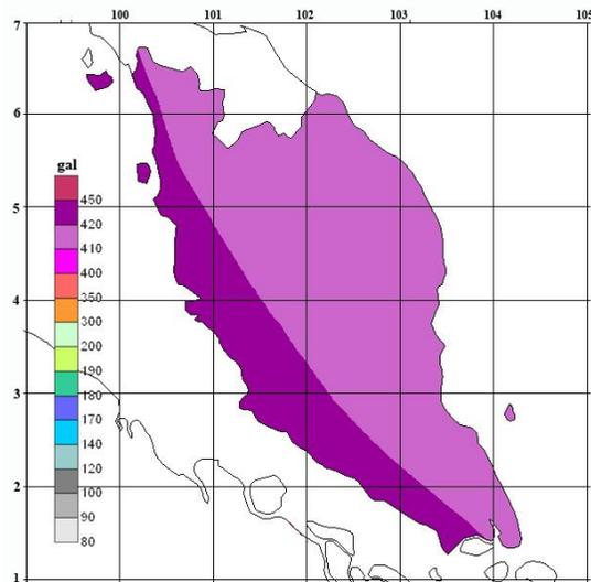
Figure 13. Probabilistic seismic hazard map of 0.2 sec spectral acceleration expected at 2% probability in 50 years on bedrock
