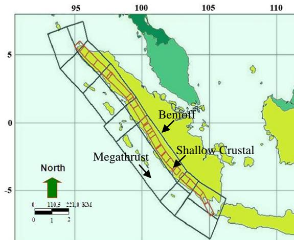
Figure 7. Seismic source zones for site location
