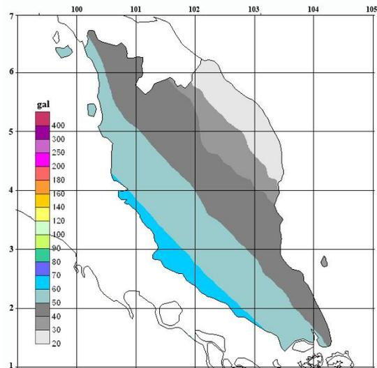
Figure 11. Probabilistic seismic hazard map of 1.0 sec spectral acceleration expected at 10% probability in 50 years on bedrock
