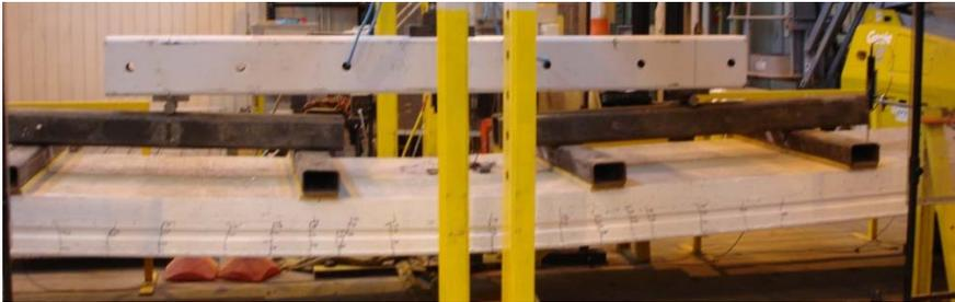
Figure 9 Flexural cracking pattern at failure for specimen SR2
