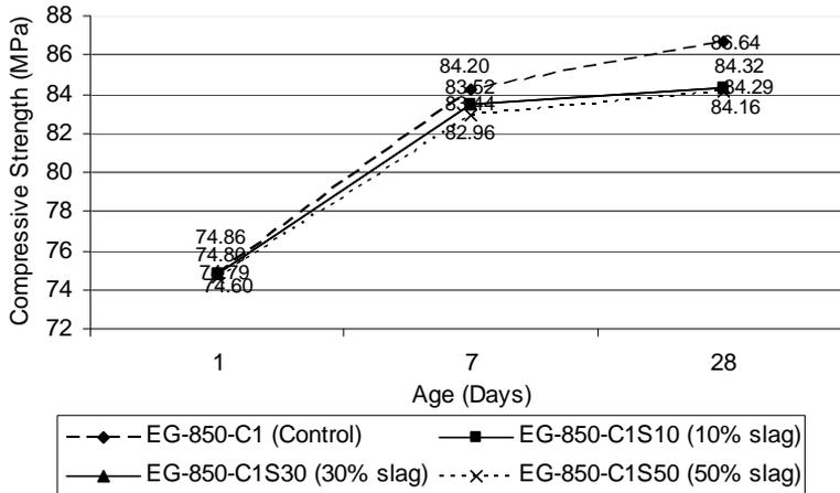
Figure 3: Compressive strength of epoxy grout with various replacement level of GGBFS as filler (epoxy:hardener:filler ratio 5:1:11)
