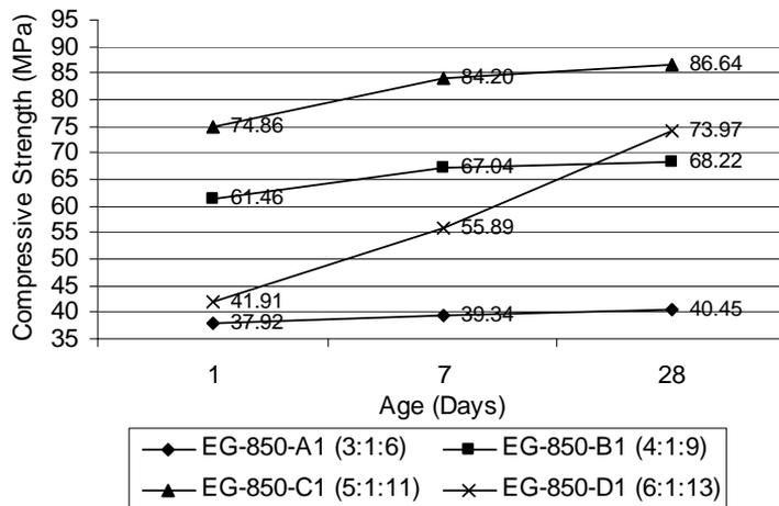
Figure 2: Compressive strength of epoxy grout with different epoxy: hardener: filler ratios at various ages
