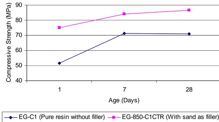
Figure 1: Compressive strength of epoxy cubes (without filler) and epoxy cubes (with filler) at various ages
