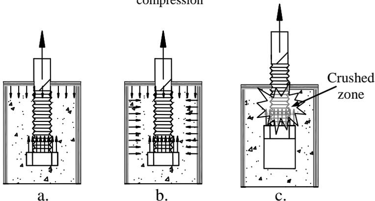
Figure 22: Crushing mechanism of specimen CS-07
