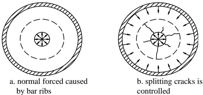
Figure 20: Confinement has controlled generation of splitting cracks
