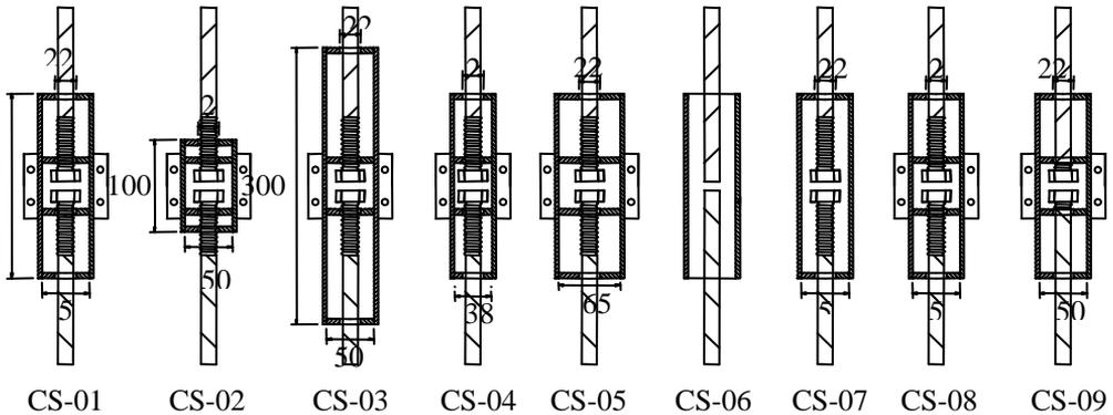
Figure 3: Proposed specimens for tensile test
