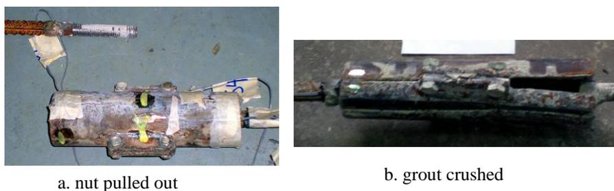
Figure 9: Failure modes of sleeves under tensile test
