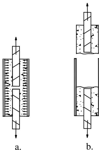
Figure 25: Split mechanism grout in steel cylinder
