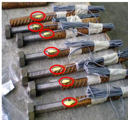
Figure 6: Installation of strain gauges on the reinforcement bar
