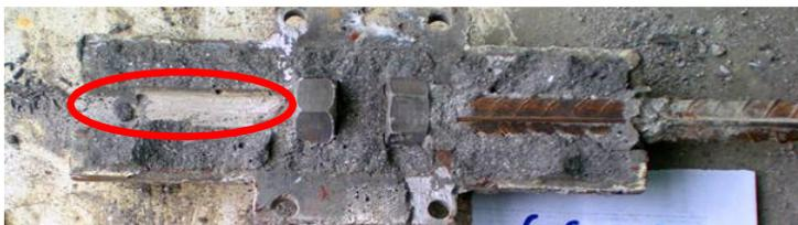
Figure13: Dusty, smooth surface Of grout due to bar slippage of specimen CS-09
