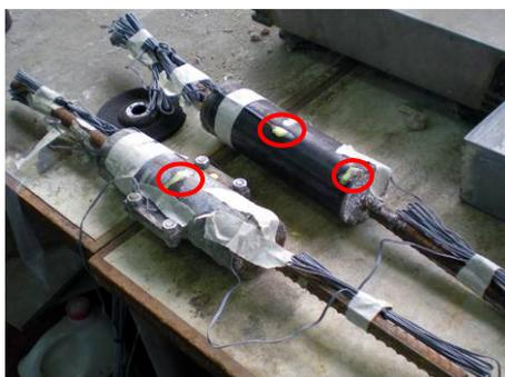
Figure 7: Installation of strain gauge on the steel sleeve
