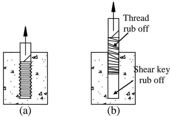
Fig. 16: Mechanism of slipped out of sleeve
