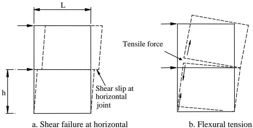
Figure 2: Types of loading for precast panel system
