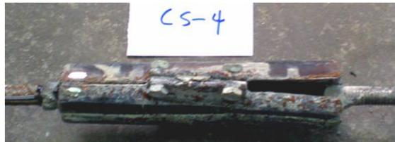
Figure 11: Dislocation of reinforcement bar with nuts on it caused one end of sleeve to split
