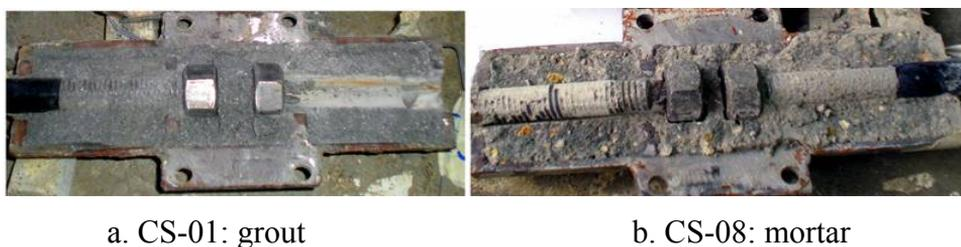
Figure 18: Comparison of bonding medium used in specimens CS-01 and CS-08
