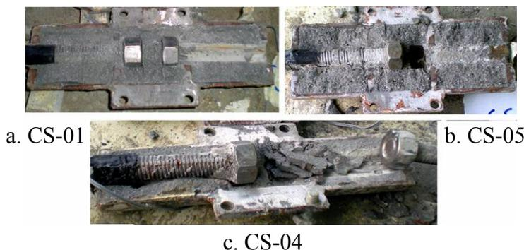
Figure 13: Failure modes of specimen CS-01, CS-02 and CS-05
