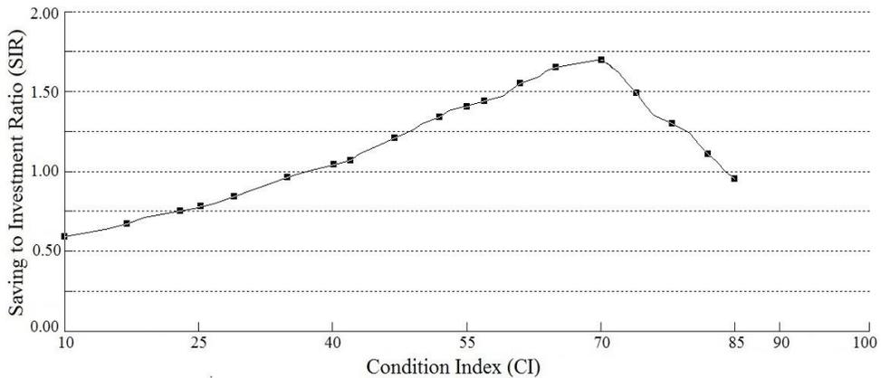
Figure 2: Optimum maintenance time and cost of cast iron pipe based on USACERL CI
