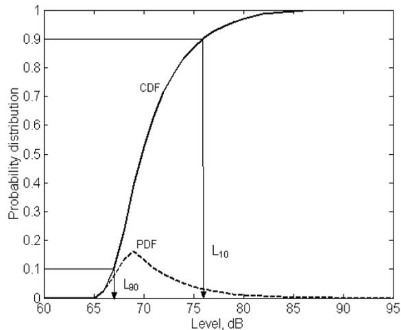
Figure 5: Temporal distribution of noise level from Excavator working full power
