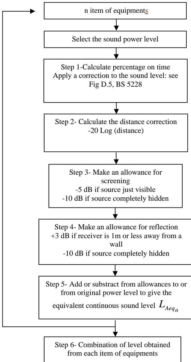
Figure 9: Flow chart for simulation of combination of concurrent activities
