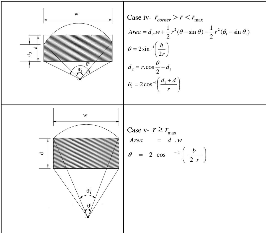
Figure 2(Continued): Calculation of possible shaded area in each case
