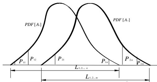
Figure 3: Division of two PDF for concurrent combination operation
