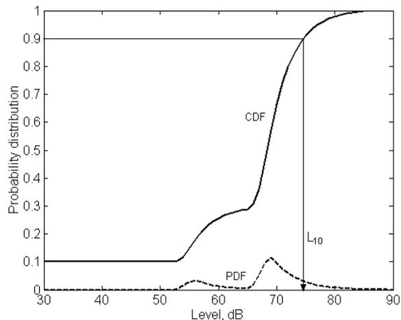
Figure 6: Temporal distribution of noise level from Excavator working with duty cycle
