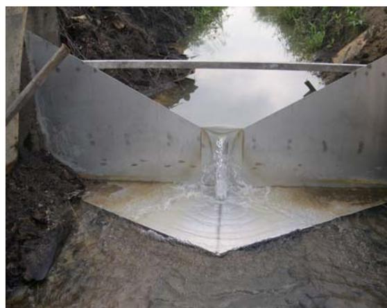
Figure 3: 120° V-notch weir
