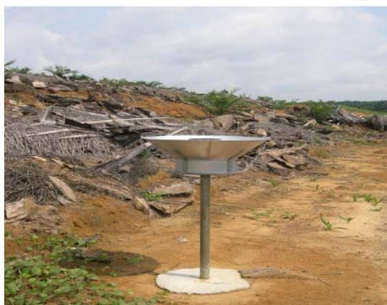
Figure 2: ONSET RG2-M automatic tipping bucket rain gauge
