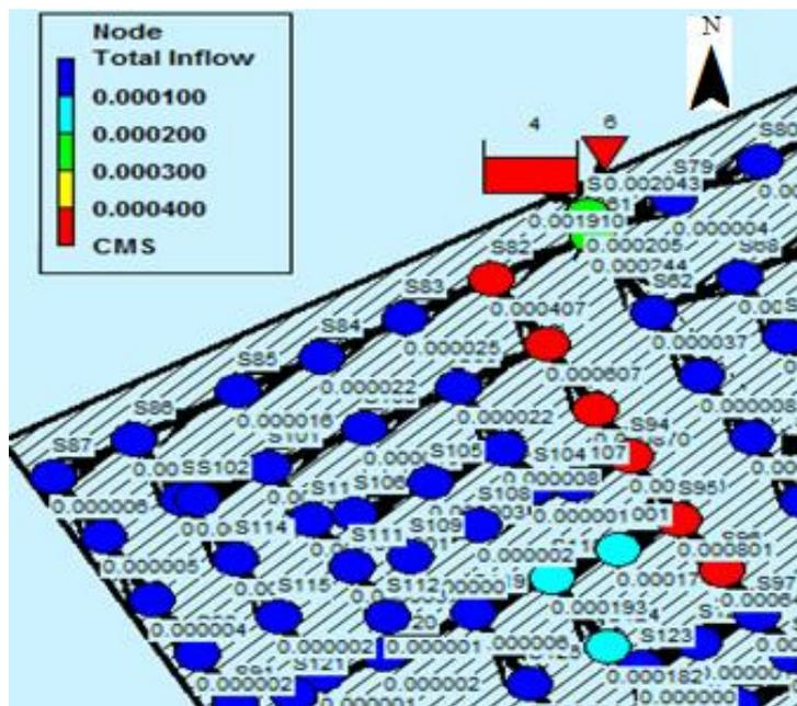
Figure 4: Total flow in sewer networks before rainfall
