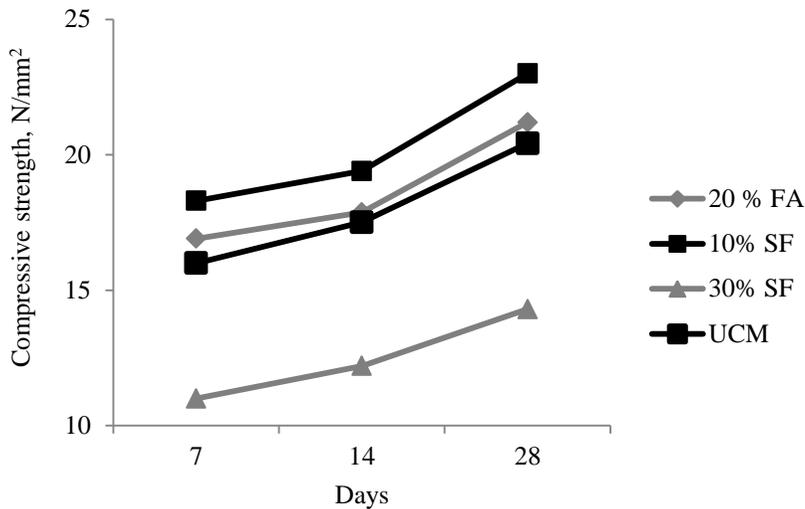
Figure7: Comparison of CS versus days for PMM and UCM
