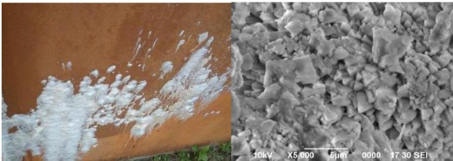
Figure 1:(a) Efflorescence on concrete wall (b) Scanning Electron Micrograph (SEM) image of efflorescence collected from the wall.
