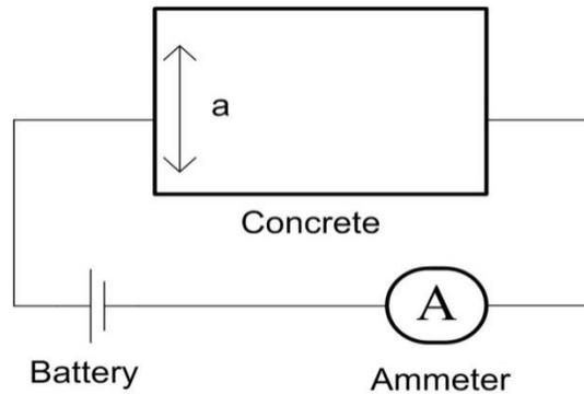
Figure 4: Basic Measure Resistivity
