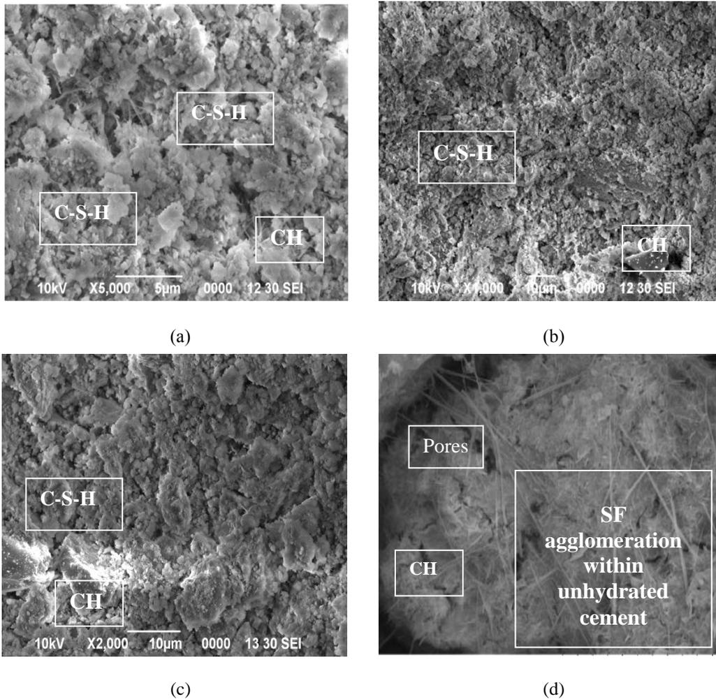
Figure 8: SEM images of (a) UCM (b) 20%FA and (c) 10%SF and (d) 30%SF samples at day 28
