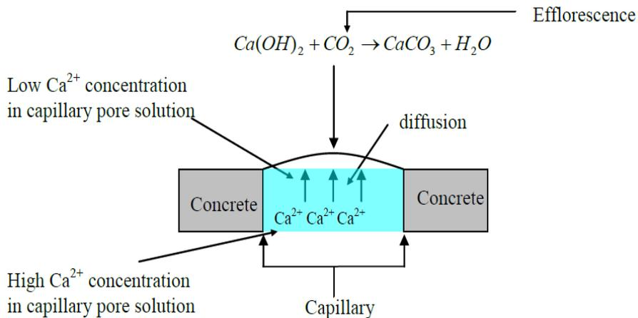
Figure 2: Schematic diagram of efflorescence from cross sectional view of concrete block.
