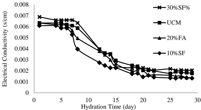
Figure 6:Electrical Conductivity of Mortar of PMM and UCM samples.
