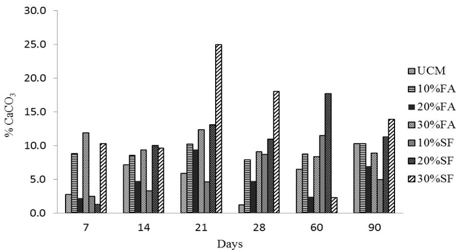
Figure 5: Comparison of Percentage (%) of CaCO<sub>3</sub> versus days for FA and SF modified mortars with Control
