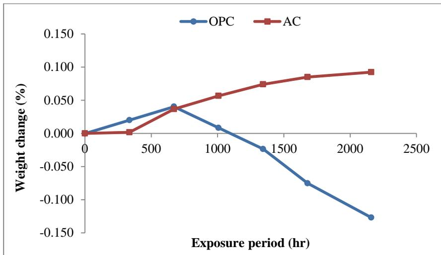
Figure 3: Mass changes in concrete cube specimens
