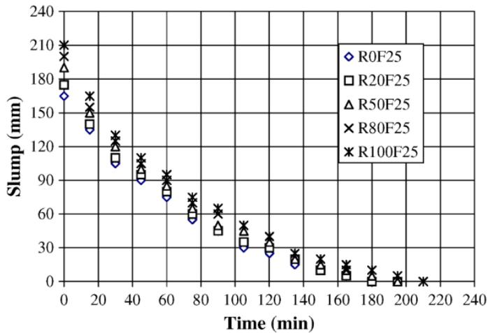
Figure 2: Changes of slump of concrete mixes with 25% fly ash with varying replacement rate of recycled aggregate, Poon *et al.* (2007)
