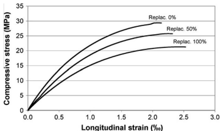
Figure 3: Stress-strain relationship of recycled aggregate concrete with varying replacement rate of recycled aggregate, Lage *et al.* (2012).
