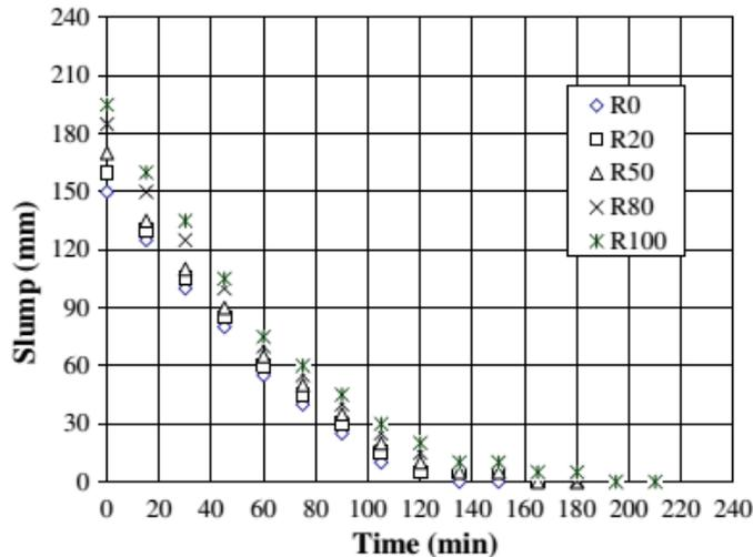
Figure 1: Changes of slump of concrete mixes without fly ash with varying replacement rate of recycled aggregate, Poon *et al.* (2007)
