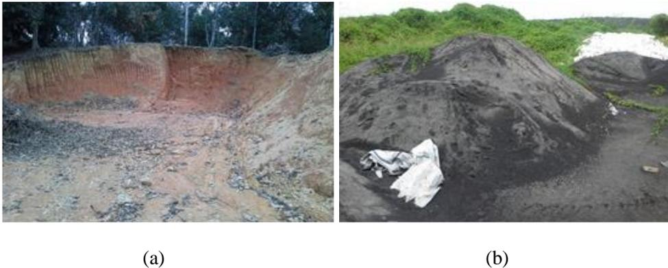
Figure 1: (a) Granite residual soil from Hulu Langat, Selangor (b) Disposal practice of POFA around the factories
