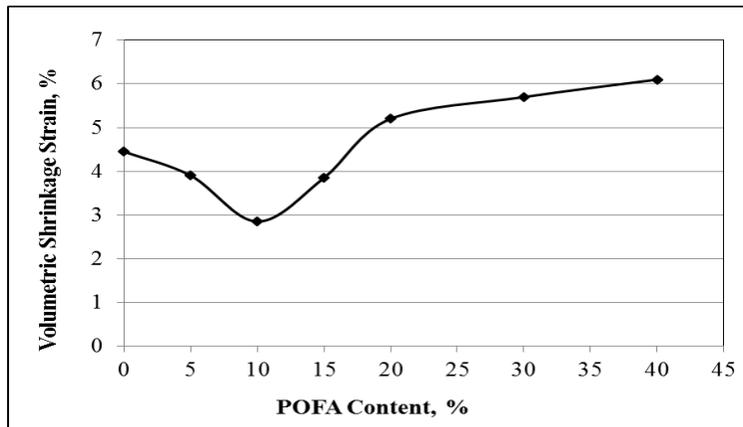
Figure 4. Variation of volumetric shrinkage strain (VSS) with POFA content
