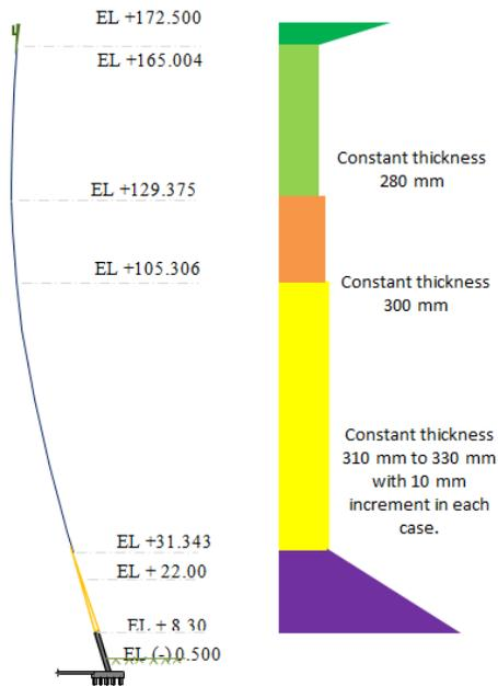
Figure. 9 Shell thickness variation model for Case 22 to 24
