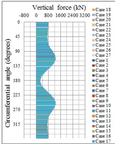
Figure 23: Variation of VFP on 4<sup>th</sup> row of piles
