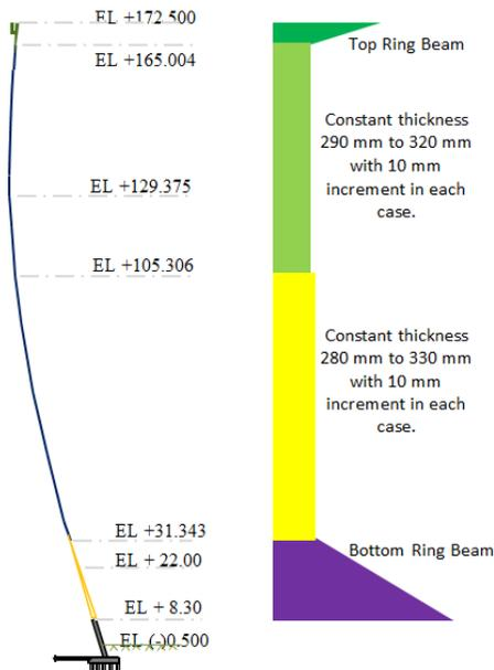
Figure. 7 Shell thickness variation model for Case 13 to 17
