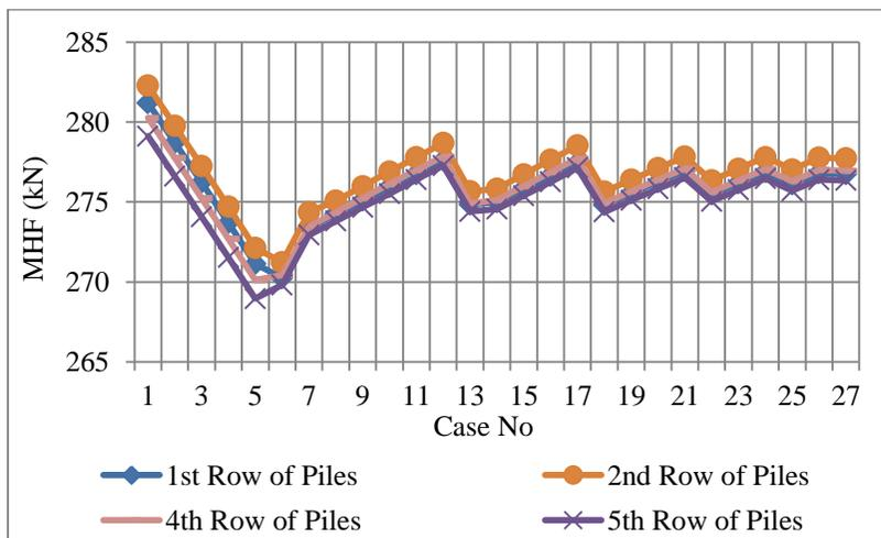
Figure 17: Variation of MHF on piles
