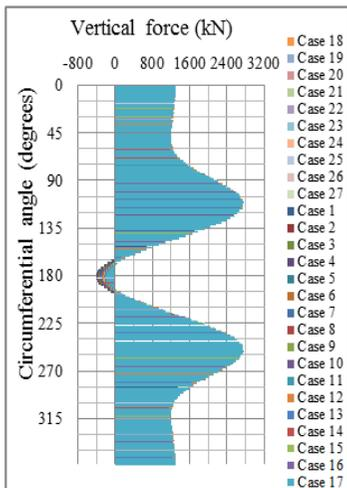
Figure 20: Variation of VFP on 1<sup>st</sup> row of piles
