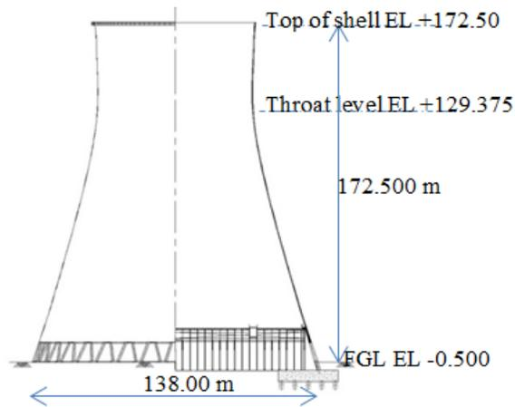
Figure 1: General Arrangement of NDCT
