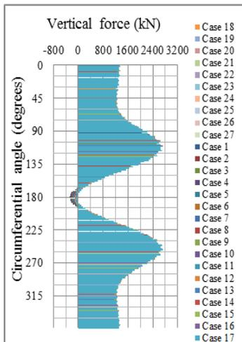
Figure 21: Variation of VFP on 2<sup>nd</sup> row of piles.
