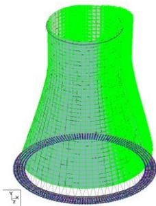
Figure 15: Wind pressure on the NDCT shell -3D view
