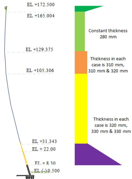
Figure. 10 Shell thickness variation model for Case 25 to 27
