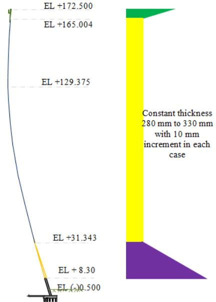
Figure. 6 Shell thickness variation model for Case 7 to 12
