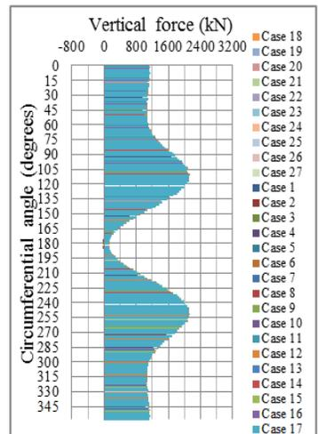
Figure 22: Variation of VFP on 3<sup>rd</sup> row of piles.
