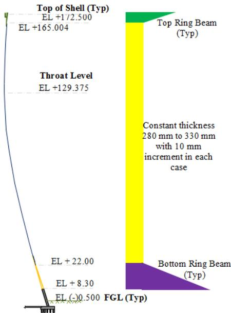
Figure. 5 Shell thickness variation model for Case 1 to 6
