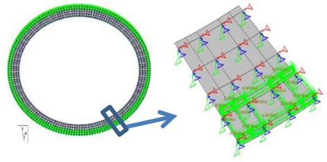
Figure 14: Vertical pressures due to soil and surcharge on the pile cap
