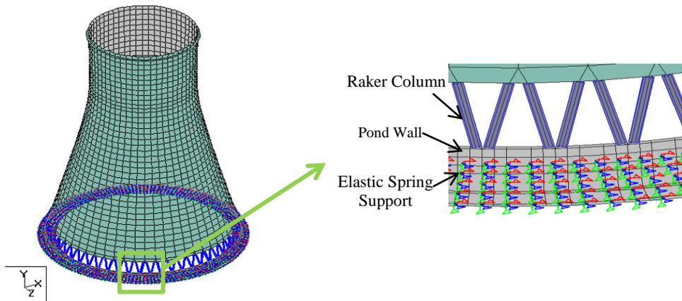
Figure 12: FEM model of NDCT Composite model
