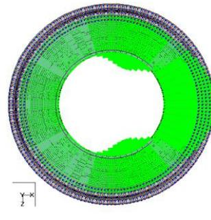
Figure 16: Wind pressure on the NDCT shell -top view
