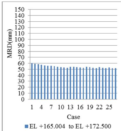
Figure 29: Variation of MRD in shell from EL + 165.004 m to EL + 172.500 m
