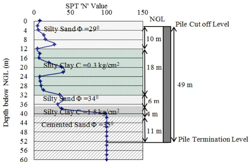
Figure 4: Variation of SPT 'N' Value the Soil Profile considered
