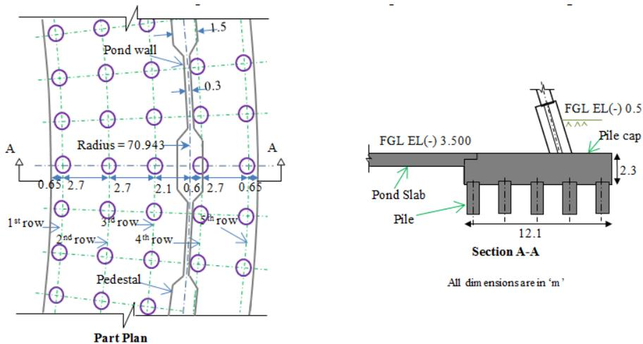
Figure 11 : Part plan & section showing piling layout
