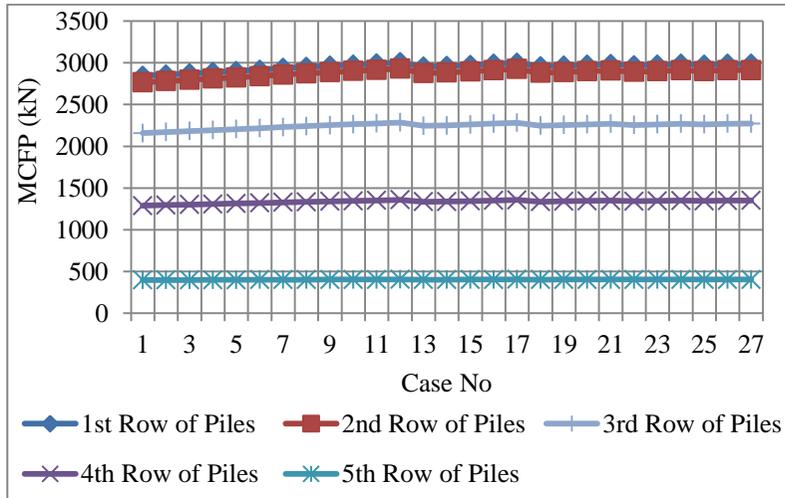
Figure 18: Variation of MCF on piles
