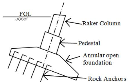
Figure 2: Annular open foundation for NDCT      Figure 3: Raker pile foundation for NDCT
