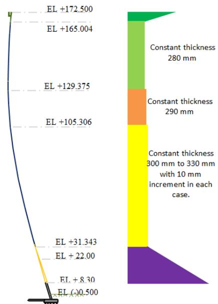
Figure.8 Shell thickness variation model for Case 18 to 21
