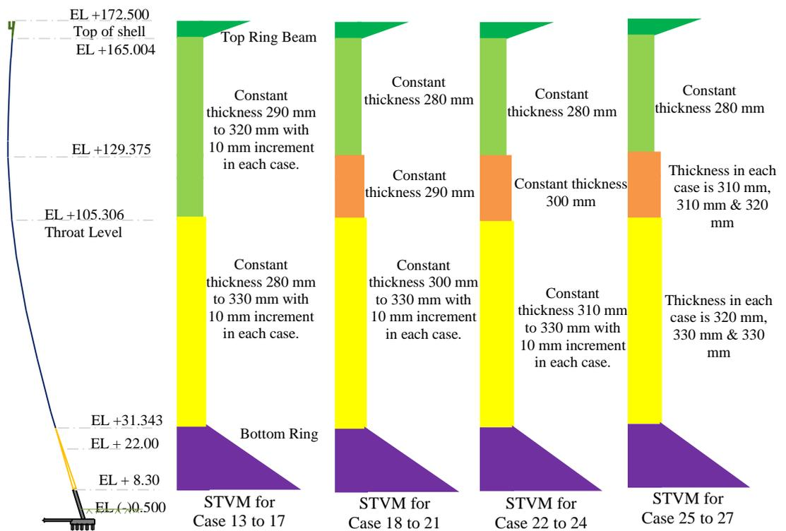
Figure 31: Best STVM's identified for NDCT resting on vertical pile foundation
