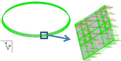
Figure 13: Lateral pressures due to soil and surcharge on the wall and pedestals
