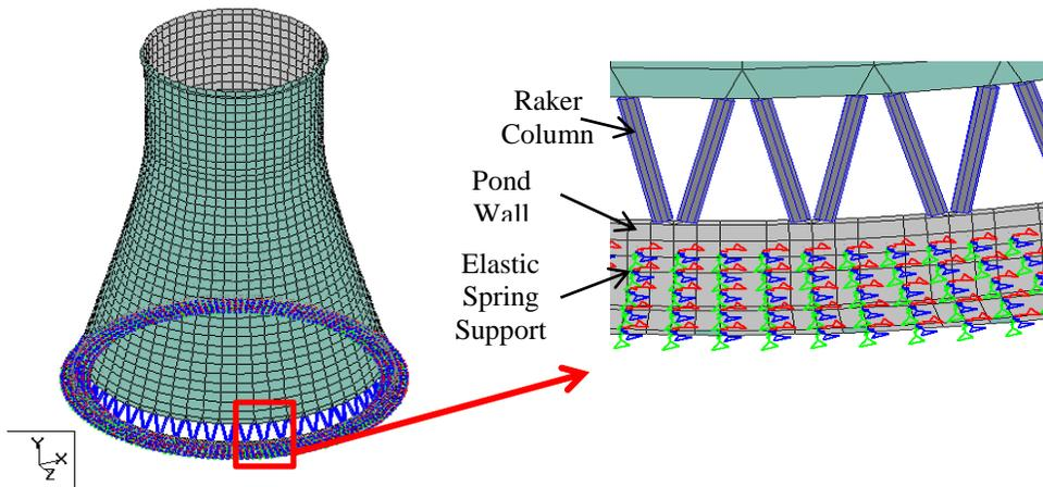
Figure 10: Finite Element Model of NDCT
