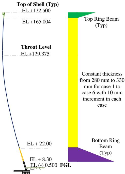
Figure 2: Shell thickness variation model for Case 1 to 6
