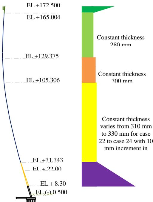
Figure 6: Shell thickness variation model for Case 22 to 24
