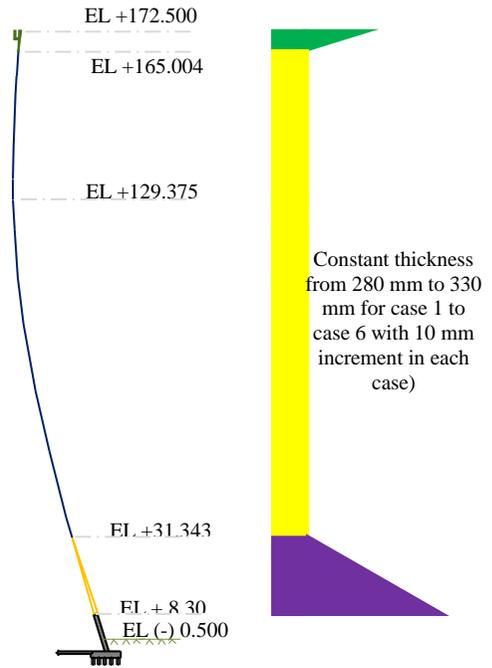
Figure 3: Shell thickness variation model for Case 7 to 12
