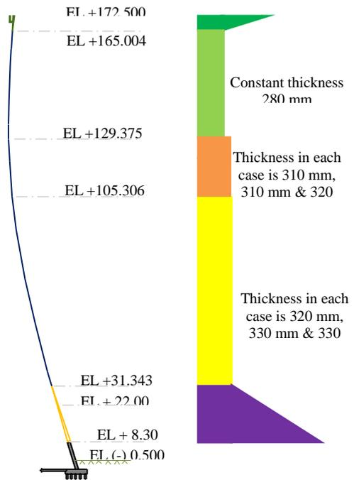
Figure 7: Shell thickness variation model for Case 25 to 27
