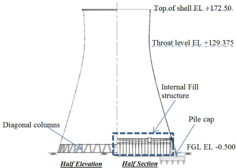
Figure 1: Natural draught cooling tower showing half elevation and half section
