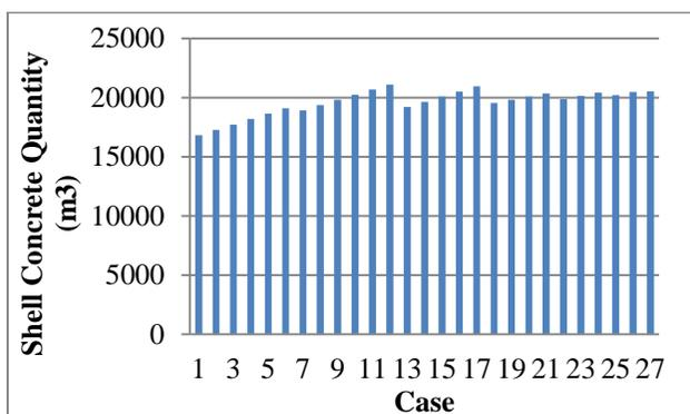
Figure 19: Comparison of Concrete quantity required for all cases 1-27
