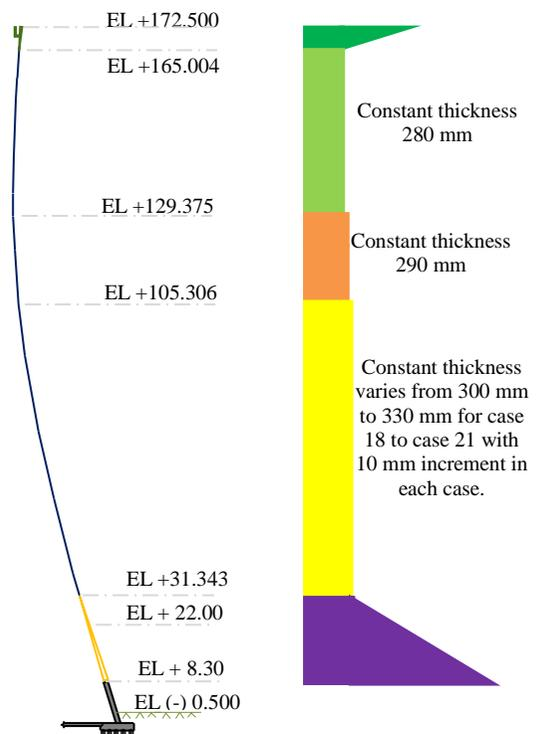
Figure 5: Shell thickness variation model for Case 18 to 21
