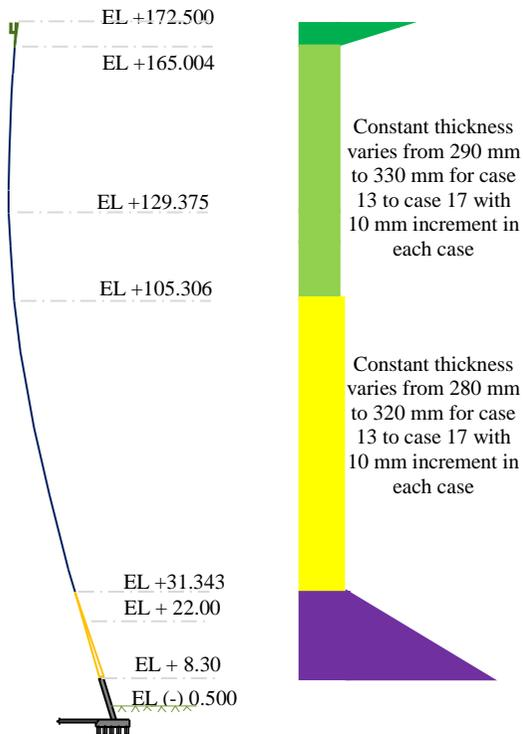
Figure 4: Shell thickness variation model for Case 13 to 17
