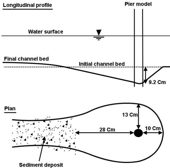
Figure 3: Dimensions of scoring hole around the pier
