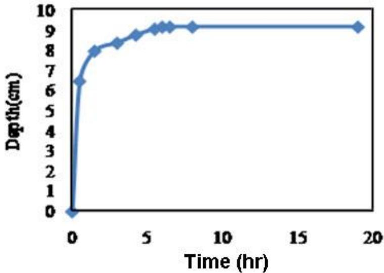
Figure 4: Development of scour depth at the pier nose
