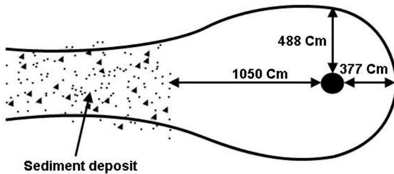
Figure 5: scouring region around the bridge pier in prototype
