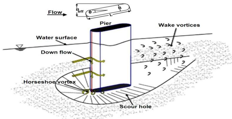
Figure 1: Schematic vortex structures around circular pier
