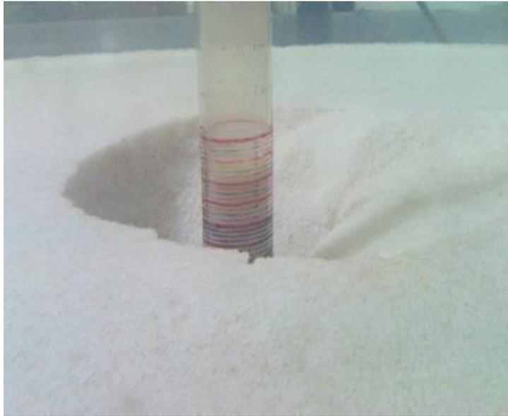
Figure 2: Experiment with the pier and scouring hole around it
