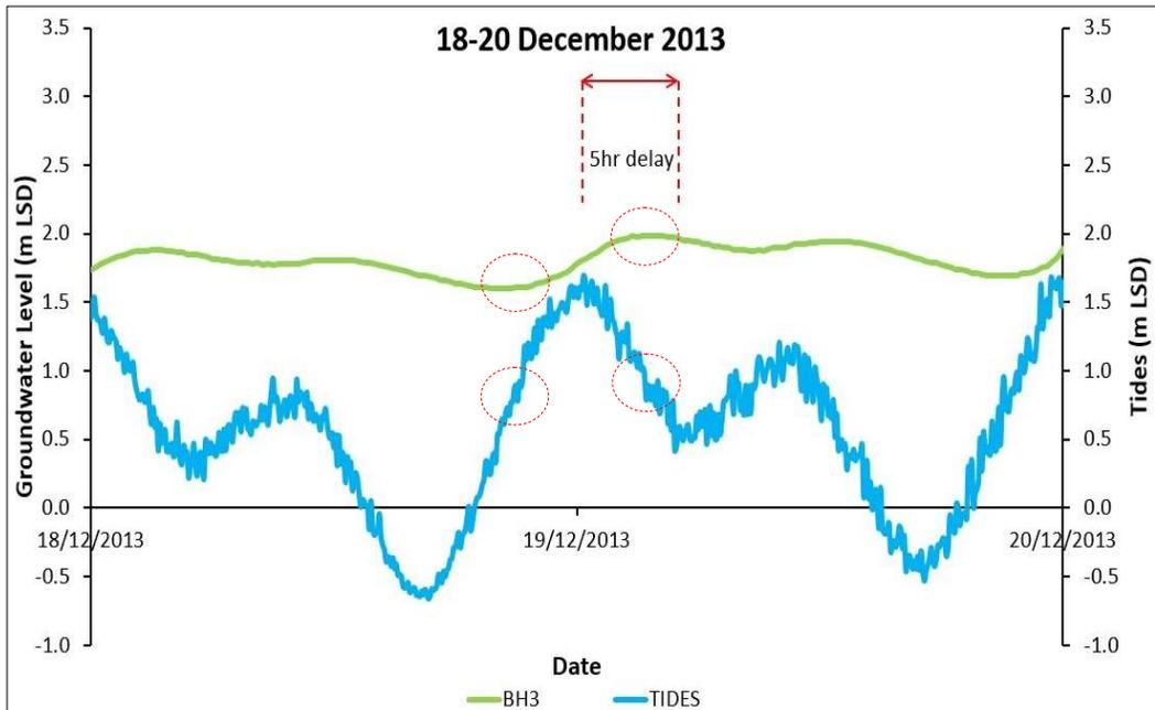
Figure 6: Relationship of Groundwater Level and Tides
