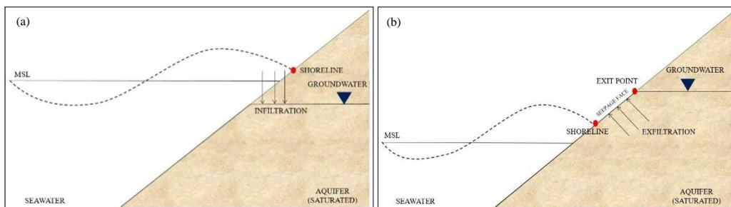
Figure 1: Beach Groundwater System. (a) Infiltration and (b) Exfiltration
