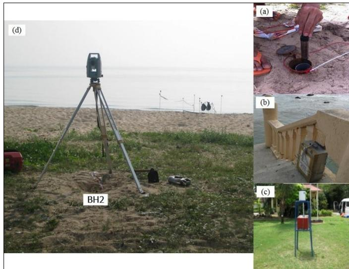
Figure 3: Fieldwork at Desaru (Othman *et al.*, 2014). (a) Monitoring Well, (b) Tide Gauge, (c) Rainfall Gauge and (d) Cross-shore Surveying
