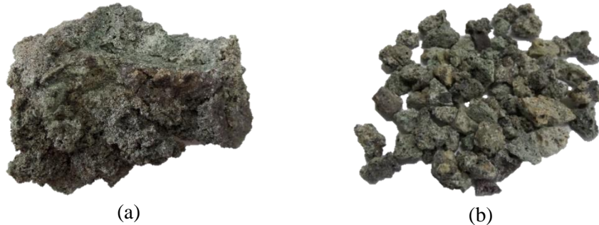
Figure 1: POC (a) Raw POC collected from palm oil mill and (b) Coarse POC aggregates after crushing and sieving
