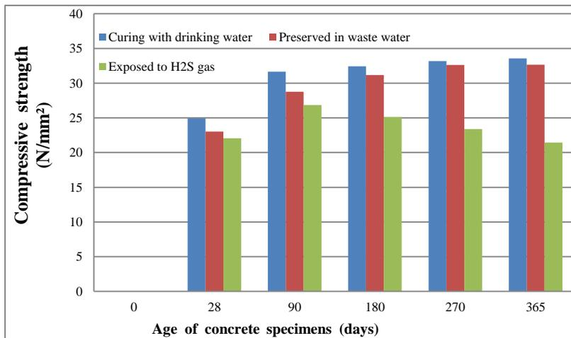
Figure 4: Compressive strength by sclerometer of concrete specimens curing in different environments.
