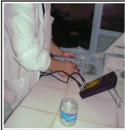
Figure 5: UPV test on the surface of prismatic concrete specimens
