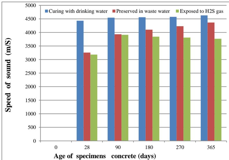
Figure 6: Speed of sound of concrete specimens cured in different environments.
