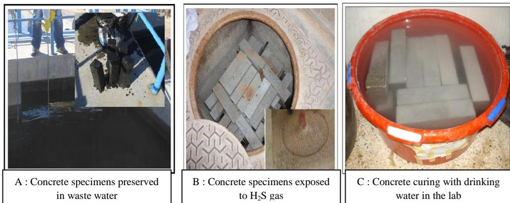
Figure 2: Concrete specimens curing in different environment
