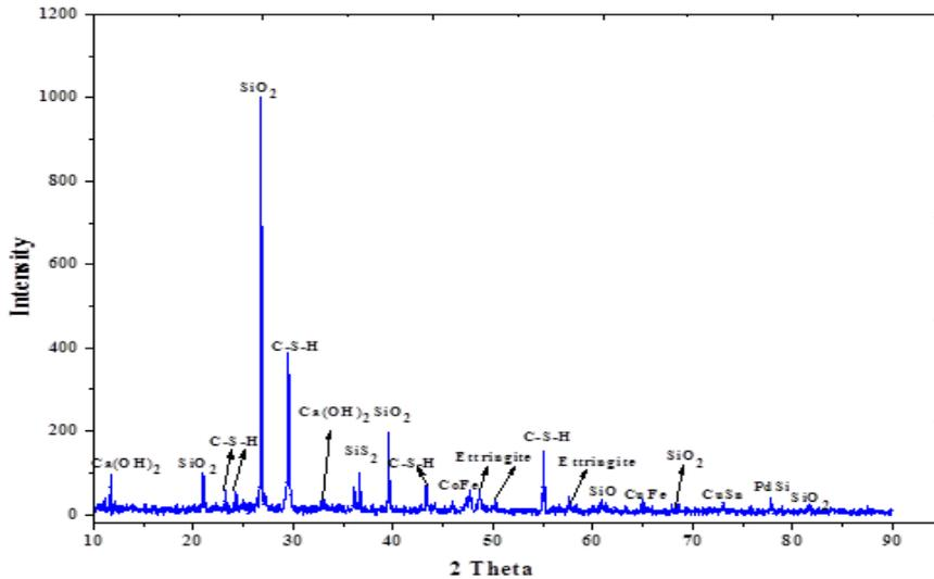
Figure 9: X-ray diffraction of specimens conserved in the waste water.
