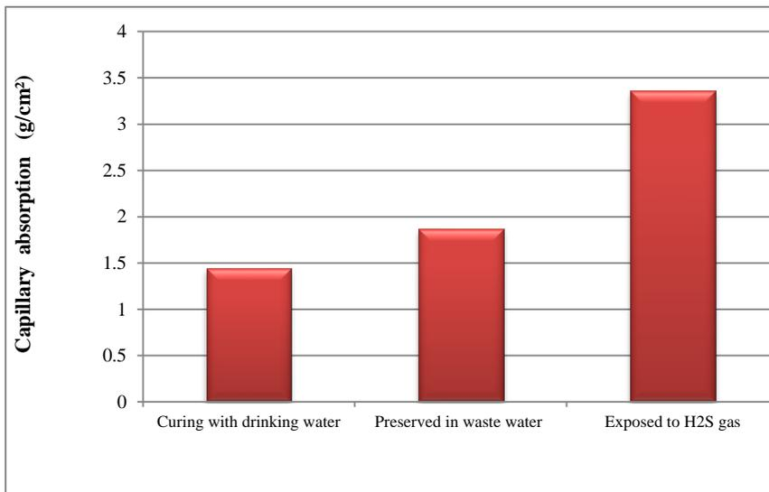
Figure 8: Capillary absorption of concrete specimens conserved in different environments.
