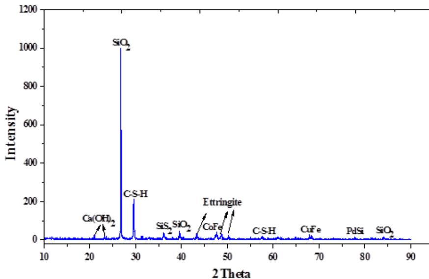
Figure 10: X-ray diffraction of specimens exposed to  $H_2S$  gas.
