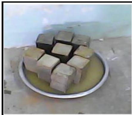
Figure 7: Capillary absorption test of prismatic concrete specimens.
