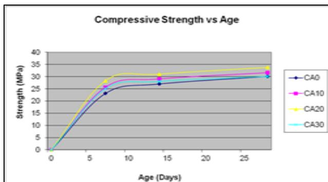
Figure 3 : Compressive Strength of Timber Clinker Aggregate Concrete without Supraccoat SP 1000.
