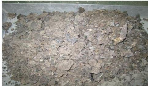
Figure 1: By-product waste - timber clinker aggregate
