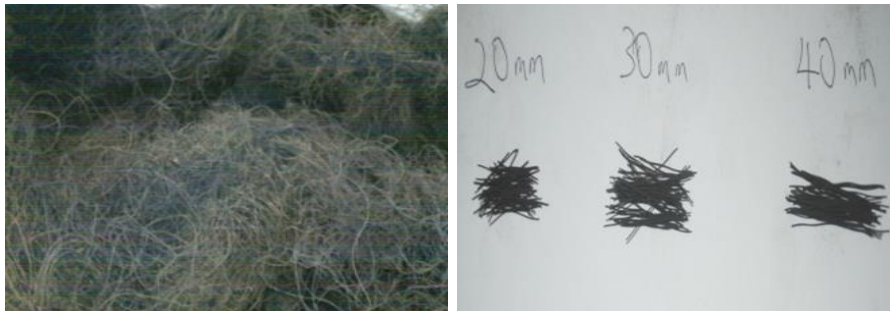
Figure 1: Recycled steel fibre before and after shredding
