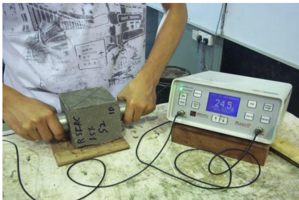
Figure 2: Testing of ultrasonic pulse velocity.
