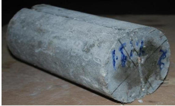
Figure 6: Concrete cylinder after splitting tensile test.
