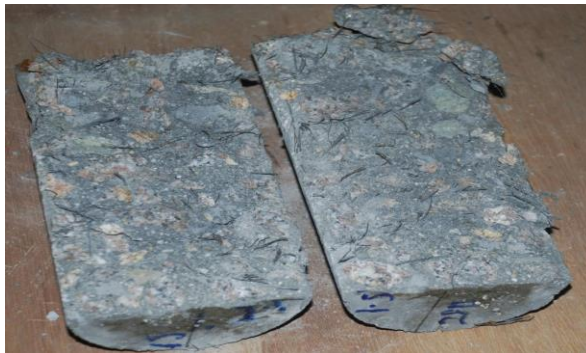
Figure 7: Distribution of steel fibre in broken cylinder.
