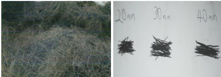
Figure 1: Recycled steel fibre before and after shredding
